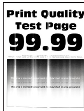
Figure 1 Vertical Light Bands
