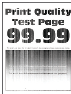
Figure 1 Vertical White Lines
