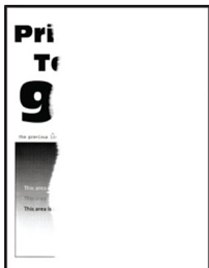
Figure 1 Text Or Images Cut Off
