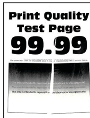
Figure 1 Folded Or Wrinkled Image
