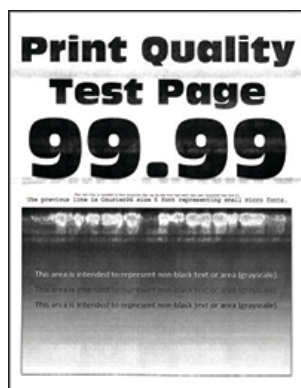
Figure 1 Horizontal Light Bands
