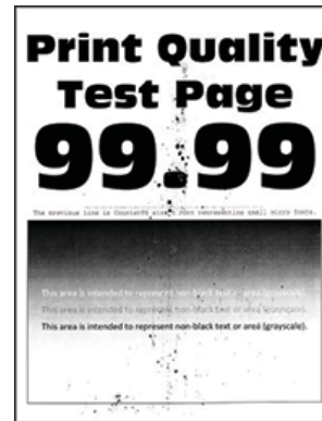
Figure 1 Mottled Print And Dots Image
