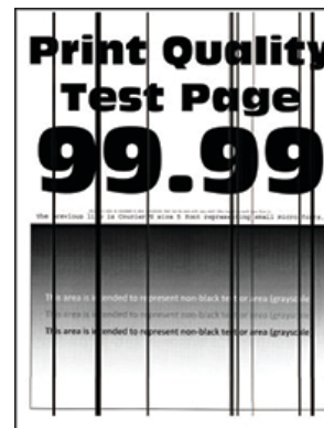
Figure 1 Vertical Dark Lines
