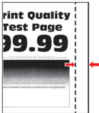
Figure 1 Incorrect Margins On Prints
