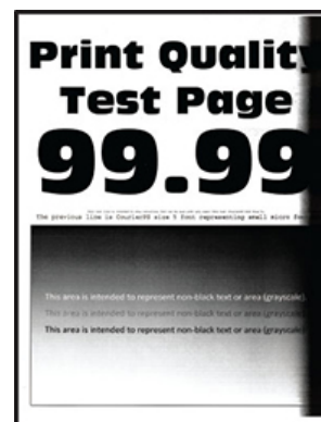
Figure 1 Vertical Dark Bands
