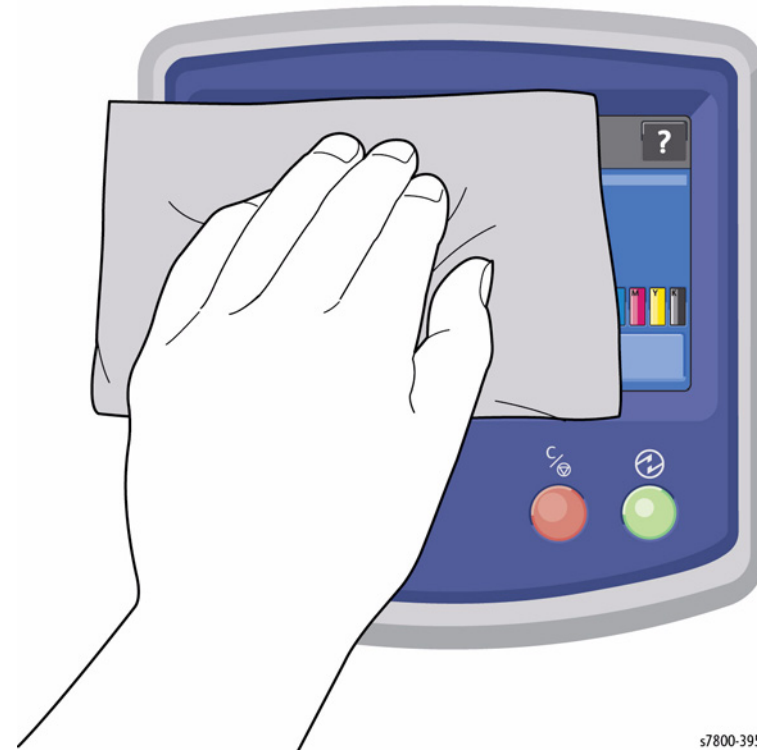
Figure 1 Cleaning the Control Panel
