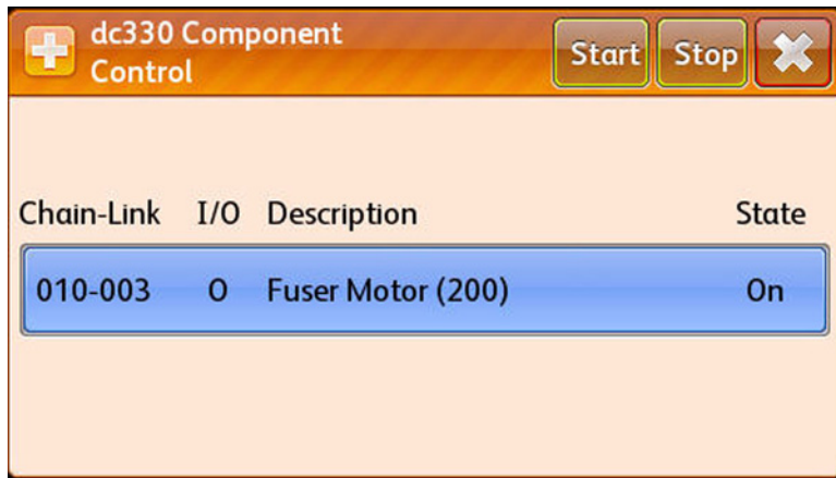
Figure 4 Starting and Stopping the Test
