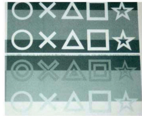
SLED Transfer Failure
