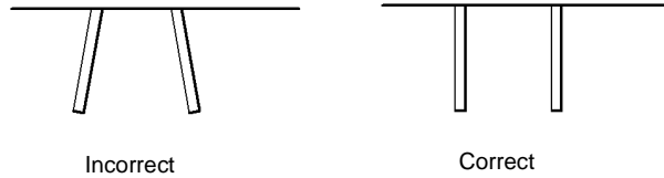
Figure 2 Correct spring bracket position.
