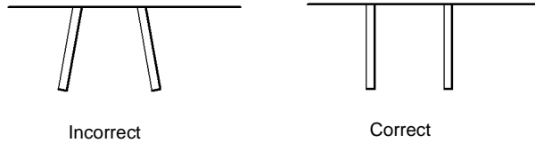
Figure 2 Correct spring bracket position.
