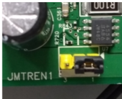
Interlock bypass enabled
