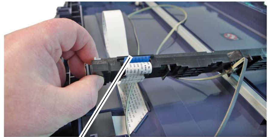
Figure 2 Contact image sensor FFC
