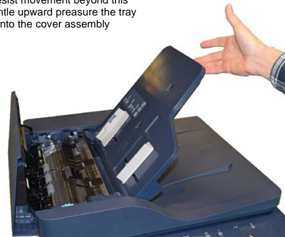
Figure 1 Lift the input tray assembly
