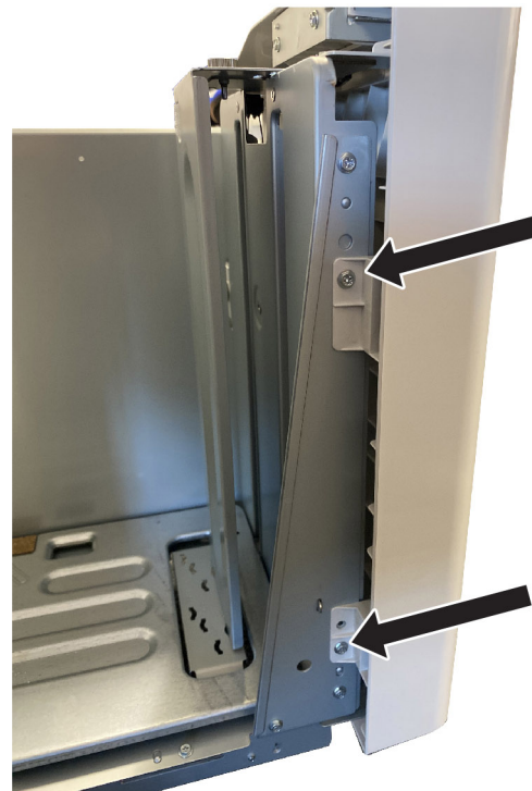
Figure 2 Removal of 2 Screws from the Left Side of the Front Cover Assembly
