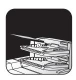
Adjust the inserter tray guide to the paper size, and load paper.
