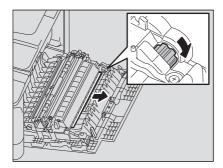
If you cannot see the misfed paper or it is difficult to remove, open the drawer in which you have loaded paper and remove it.
