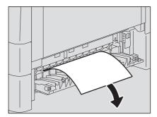
4 If it is difficult to find or remove the misfed paper, open the drawer of the Paper Feed Unit.
