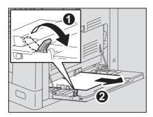
2 Check beneath the transport guide inside of the side cover. Check if any paper is misfed under the transport guide behind the transfer unit. P.153 "Paper misfeeds inside of the side cover"
