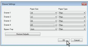
**Drawer 1** — Select the size of paper that is loaded in the Drawer 1. The paper type for the drawer is fixed to [Plain].
