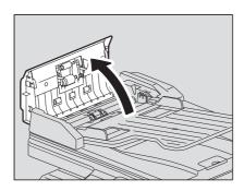
Open the transport guide and remove the original.
