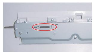
Remove six screws, and remove the lower paper guide support plate.
