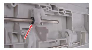
9) Slide the manual feed separation shaft in the arrow direction, and remove it from the fixing plate.
