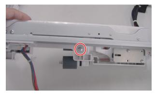
Remove the screw, and remove the pickup solenoid (Be careful of the spring.)
