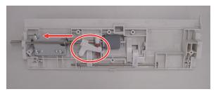
6) Remove the pressure spring.
