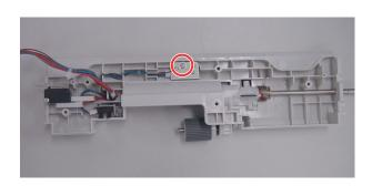
6) Remove the screw, and remove the paper empty sensor.
