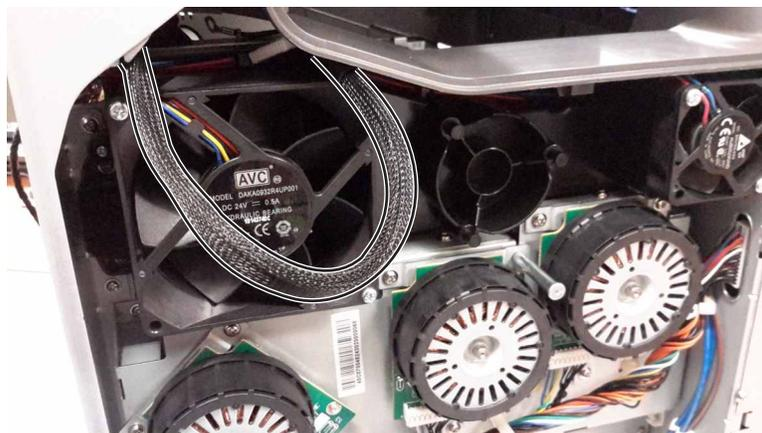
**7** Route the cable to the rear of the printer.
