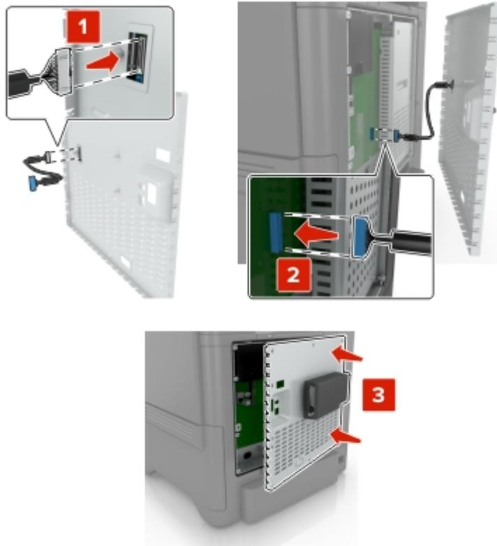
7. Reattach the controller board access cover.
