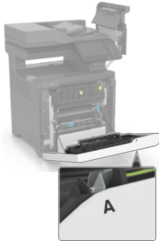
6. Remove the used transfer module.
