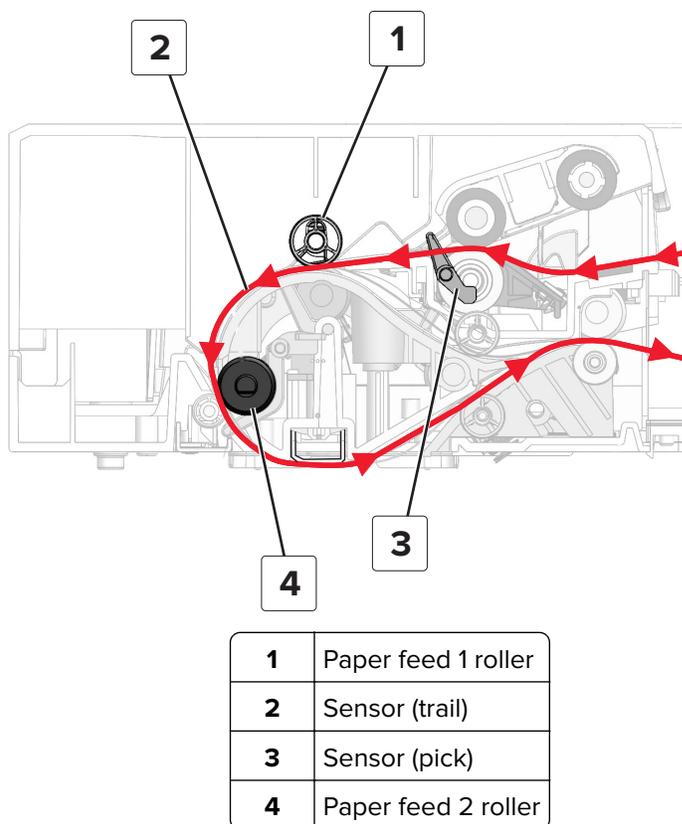
After passing through the pick assembly, the document actuates the sensor (pick). Actuating the sensor determines that this side is the first side of the document to be scanned for a two-sided scan job. The sensor (pick) triggers a count to track the position of the document between the sensor (pick) and the paper feed 1 roller. The count is generated by the encoder on the transport motor.
