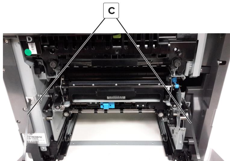
**4** Remove the screw (C) securing the ground cables.
