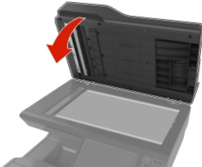
6. Open the scanner cover to check if the ADF scan pad is properly attached to the cover.
