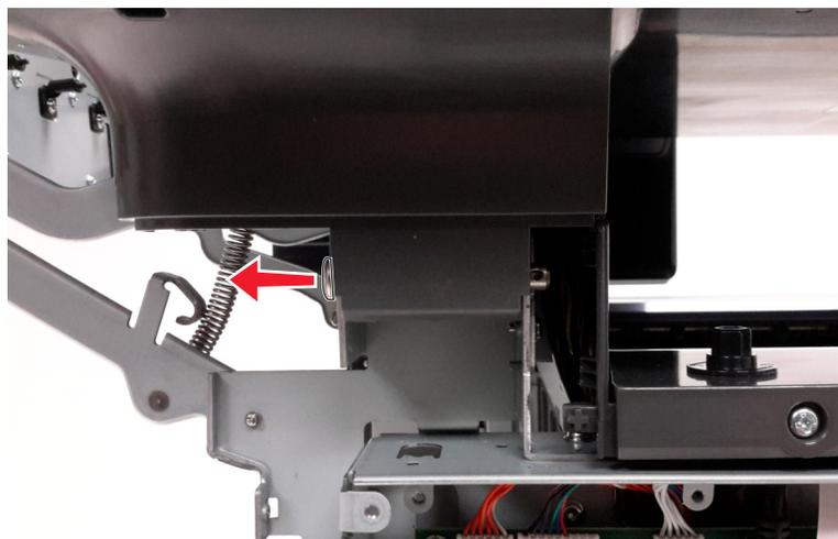
**Installation note:** Use the longer pin on the left hinge.
