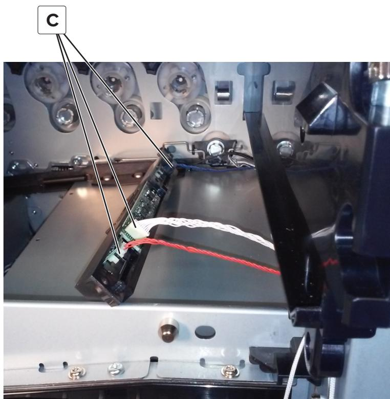
**Installation note:** Remove the protective tape covering the sensor lenses before installing the sensor assembly.
