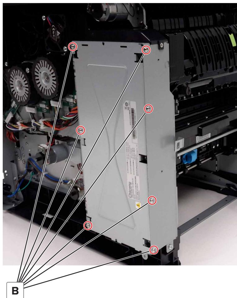
5 Disconnect the two cables (C), and then remove the LVPS.
