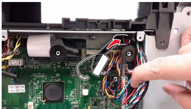
**6** Route the cable to the side of the printer.
