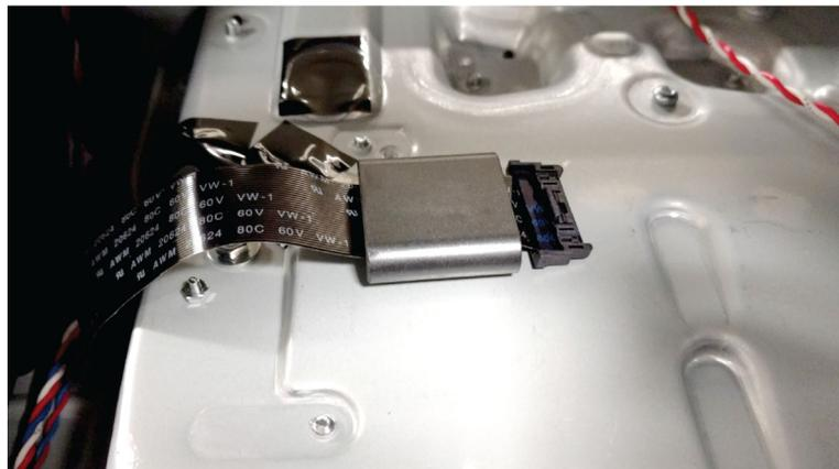
10 Route the cable through the frame and to the left side of the printer.
