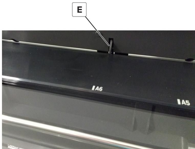
**4** Close the ADF, remove the ADF tray, and then open the ADF top cover.
