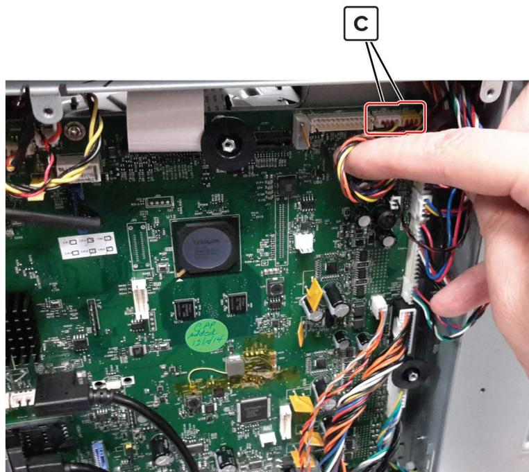
**12** Route the cables through the frame and to the left side of the printer.
