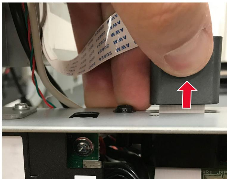
**Note:** Pay attention to the routing of the cable before releasing the cable from the frame.
