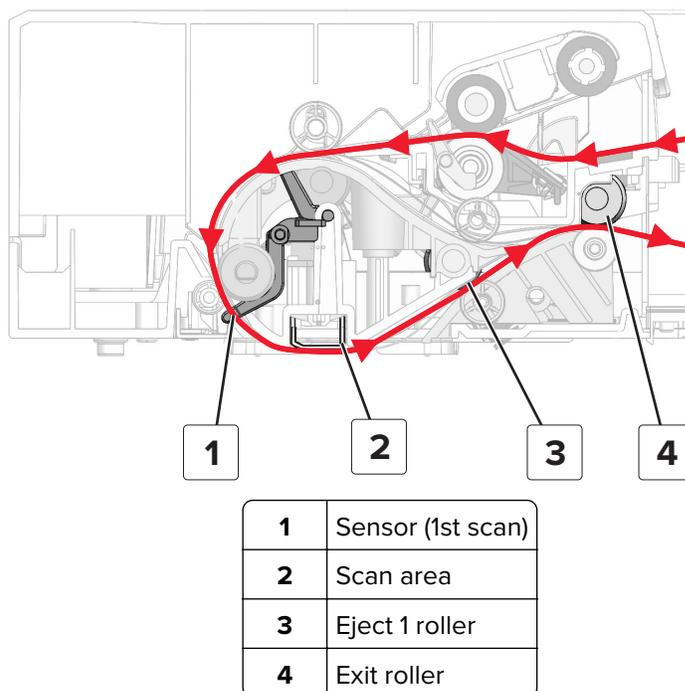
After a predetermined count, the scan document reaches the scan area and the image acquisition process is initiated. While scanning the document, the sensor (1st scan) is polled to determine if the trailing edge of the document has reached the sensor.
