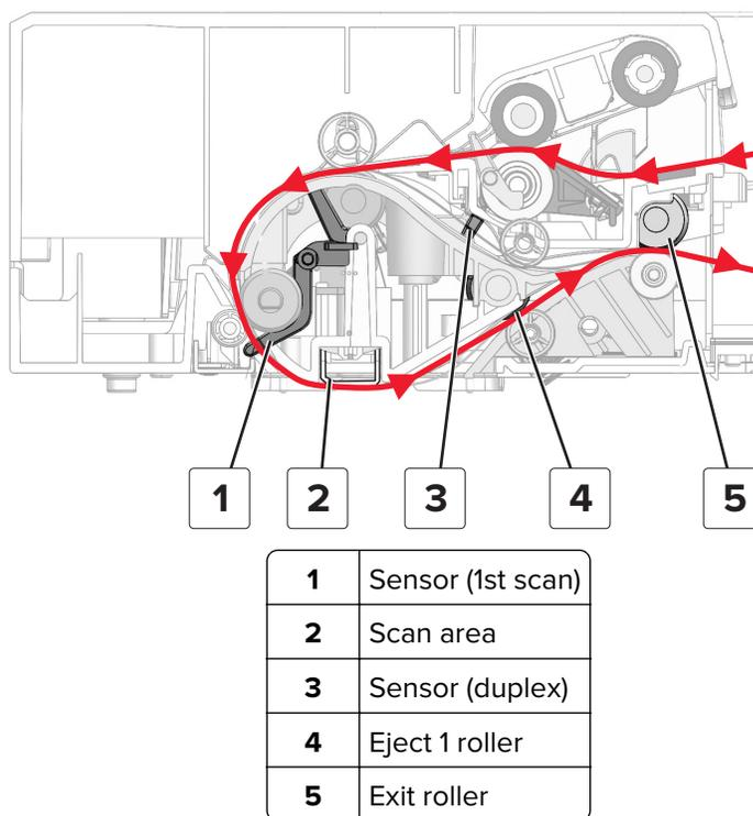
For a two-sided job, the transport motor counterrotates when the trailing edge of the scan document reaches the reverse point. The exit roller (13) pulls the document back into the ADF. The roller then moves the document to the sensor (duplex). When the sensor (duplex) (11) is actuated, this indicates to the ADF that the side of the document to be scanned is its second side.
