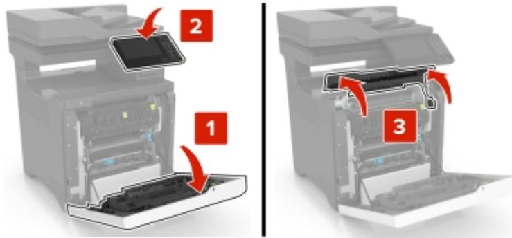
3. Remove the used fuser.
