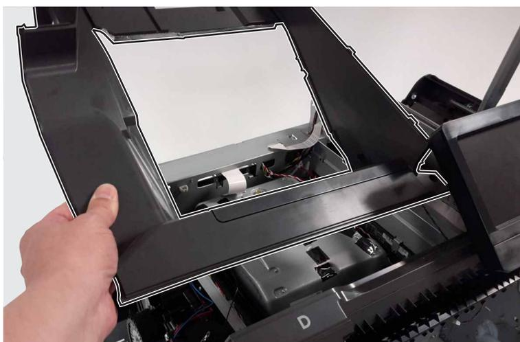
**Installation note:** Make sure that the cables are properly routed before replacing the top cover.
