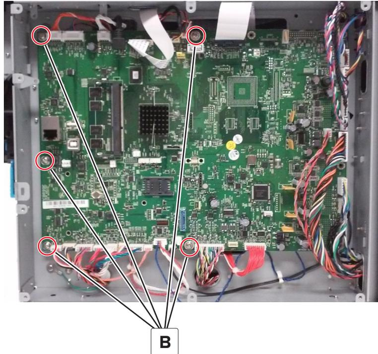
**Installation note:** After the new controller board is installed, perform printer configuration restoration. See [“Restoring the printer configuration” on page 342](#).
