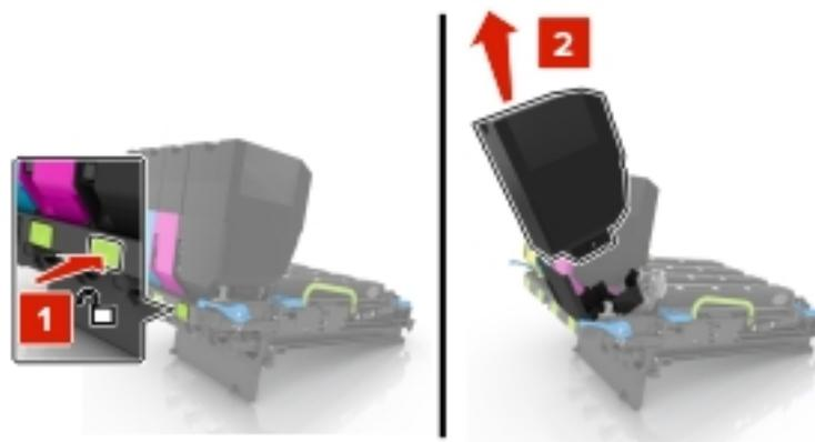
5. Remove the used imaging unit.
