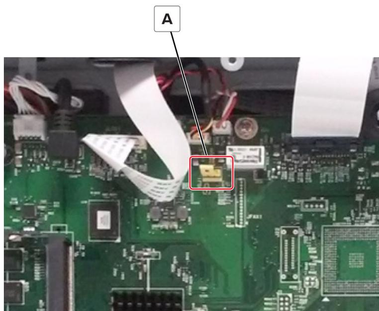
**4** Move the jumper to cover the middle and exposed prongs.
