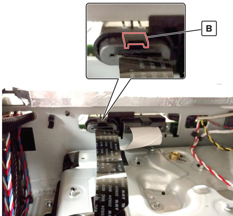
9 Pull the cable through the retainer.
