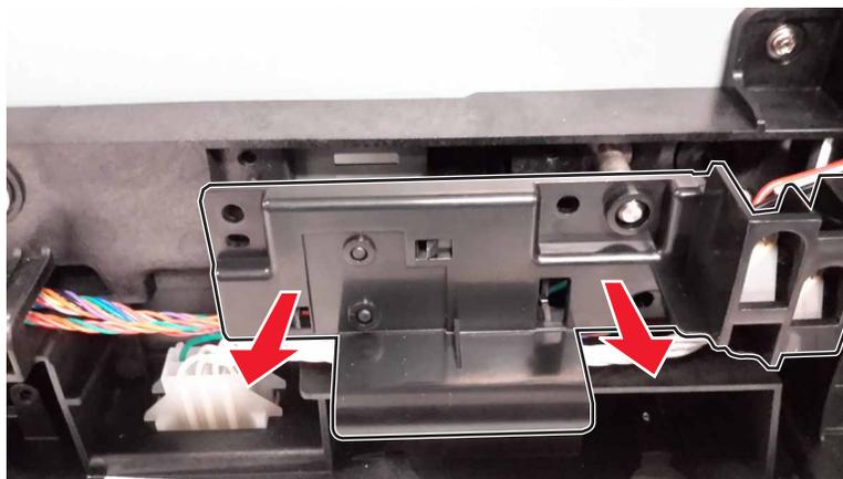
**7** Disconnect the sensor cable (B).
