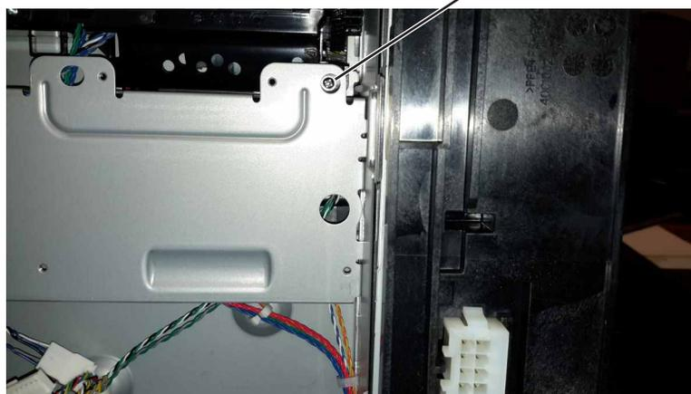
**4** Remove the biasing screw (B).
