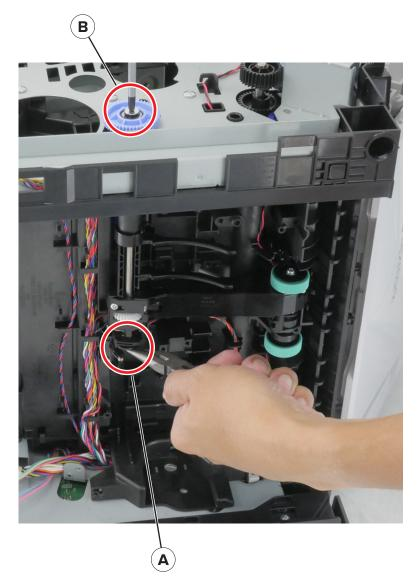
8 Pull out the pick roller assembly clutch, and then cut the cable to remove it.Installation note: Route the cables as shown.
