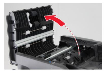
**2** Remove the ADF separator roller.
