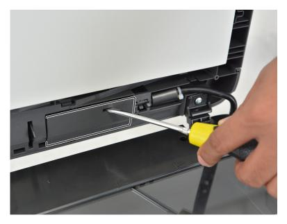
**3** Disconnect the two cables (A).
