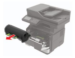
**3** Remove the used imaging unit.
