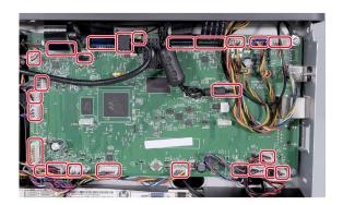
**4** Remove the five screws, and then remove the controller board.
