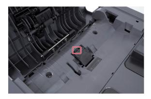
**Installation note:** Do not lose the spring under the ADF separator pad.
