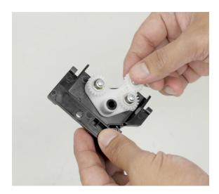
**b** Align the tab on the housing to the notch in the frame, and then install the duplex swing arm assembly.
