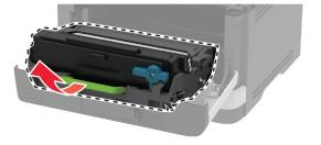
**3** Twist the blue latch, and then remove the toner cartridge from the used imaging unit.
