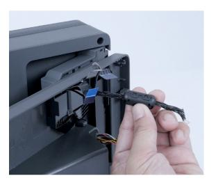
Release the three latches, and then remove the fax card.
