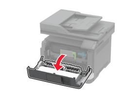
2 Remove the used imaging unit.
