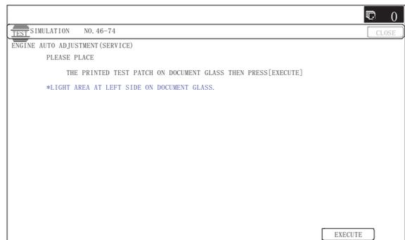
The adjustment (step 1) is automatically performed and the check patch image is printed out.
