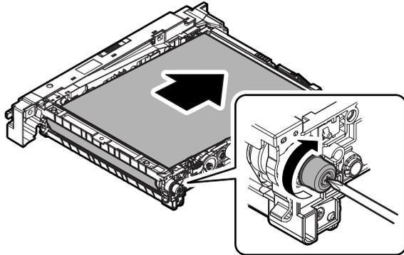
NOTE: To install or remove the primary transfer unit, hold the grip.
