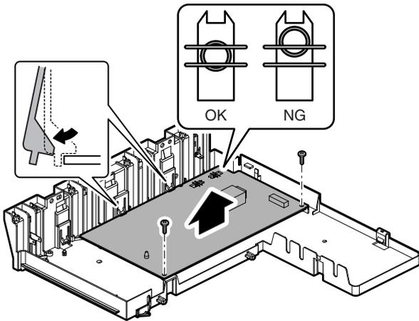
NOTE: When installing the PWB, check to confirm that there is no shift between the PWB terminal and the terminal on the MC PWB holder side.
