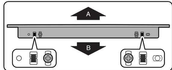
The standard fixing position is the middle of the marking scale. Change the position according to the situation.
