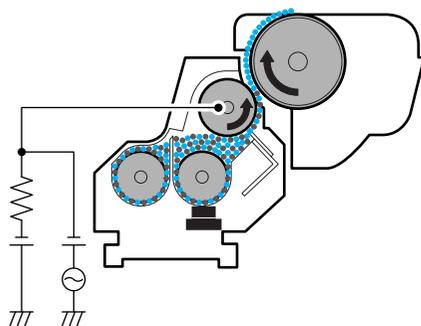
Toner and carrier in the developer cartridge are mixed and transported by the stirring roller.
