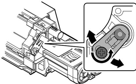
Repeat procedures 3) - 6) until the developing roller main pole position comes to the specified range.
