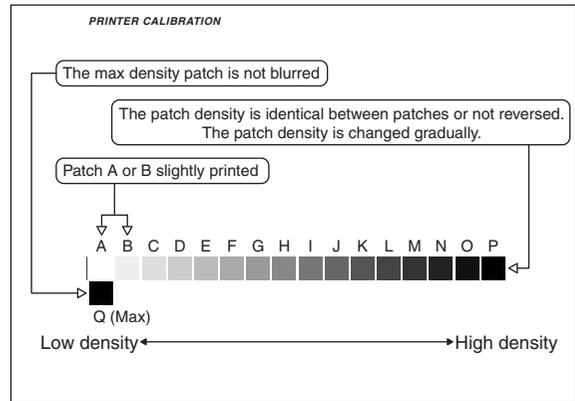
The print density must be changed gradually from the lighter level to the darker level. The density changing direction must not be reversed.
