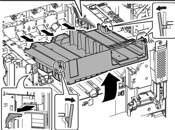
NOTE: When installing, engage the rear side of the high voltage PWB holder unit first, and then lower the front side to engage.
