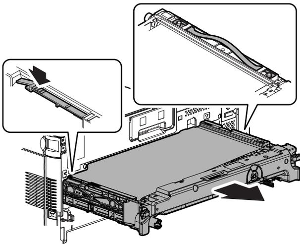
NOTE: When the primary transfer unit is removed, place several sheets of paper on the drum cartridge in order to protect the drum from being exposed.
