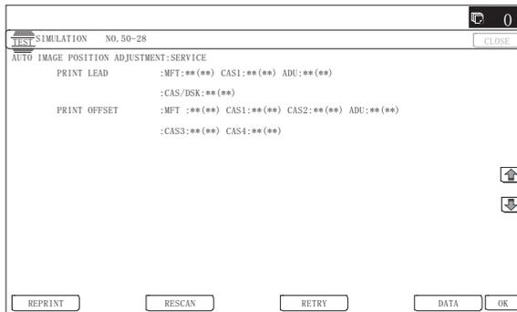
NOTE: When an error occurs in the automatic adjustment of SIM50-28, place white paper on the adjustment pattern and perform the adjustment.
