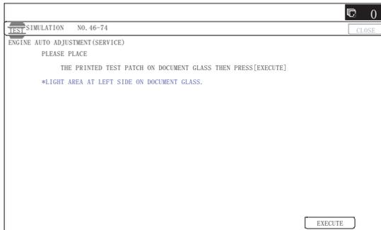
The copy density and gradation adjustment is automatically executed and prints the check patch image.
