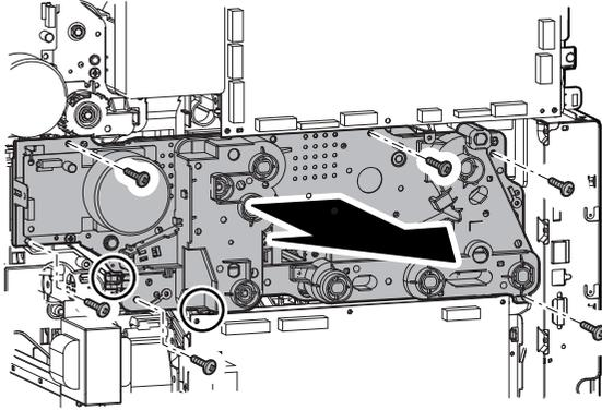
NOTE: When placing the main drive unit, place so that the motor side comes down or place on an open box so that no load is applied to the gear inside the unit.
