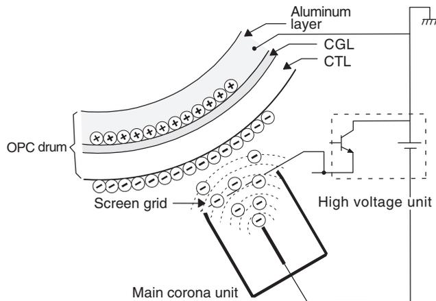
The screen grid is attached to the main charger unit, and the OPC drum is charged at a voltage which is virtually the same as the voltage applied to the screen grid.
