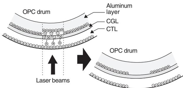
When laser beams are radiated on the OPC drum CGL, positive and negative charges are generated.
