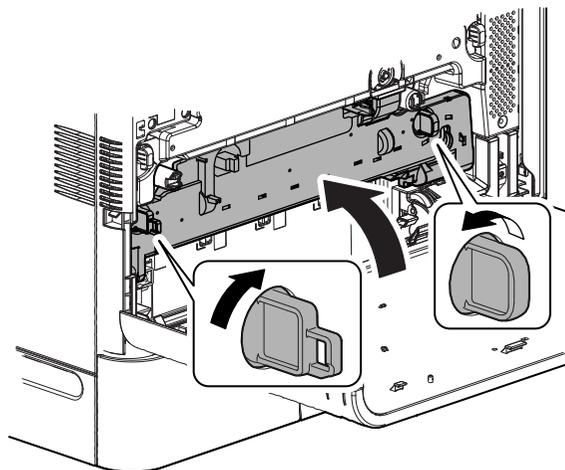
14) Install the waste toner box, and turn the lock lever to the left until it stops to lock the waste toner box.
