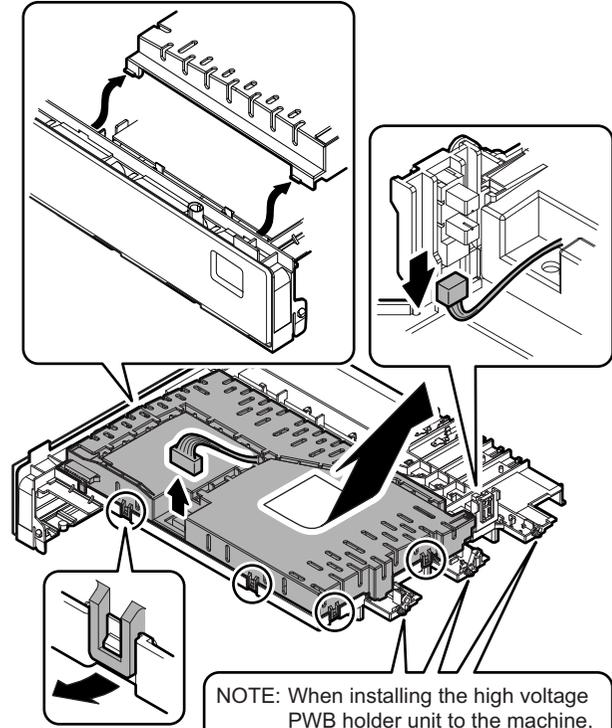
NOTE: When installing the high voltage PWB holder unit to the machine, check to confirm that there is no deformation or tilt of the terminal.
