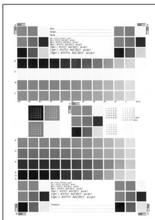
The print density must be changed gradually from the lighter level to the darker level. The density changing direction must not be reversed.
