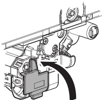
13) Close the drum positioning plate unit, and put the lock lever upright to lock.
