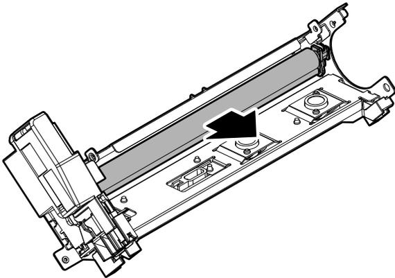
9) Remove the oil roller bearing. Remove the oil roller and the cleaning roller.
