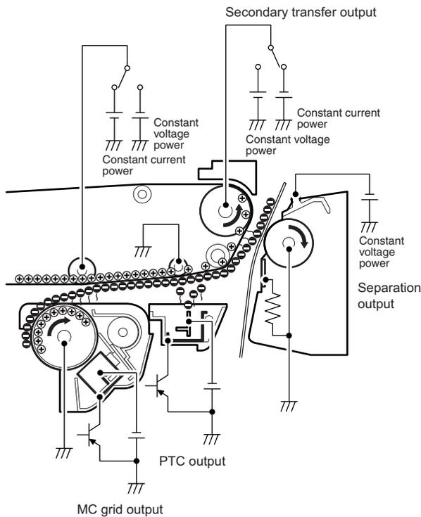
Toner images on the OPC drum are transferred onto the primary transfer belt by applying a high positive voltage to the primary transfer roller.
