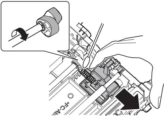
**NOTE:** Do not remove the spring of the roller separation link.
