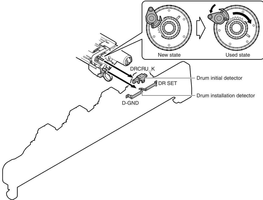
In the OPC drum positioning unit, there is a contact to detect installation of the OPC drum. If there is no OPC drum installed, it is detected and the message is displayed on the operation panel to show that there is no OPC drum installed.
