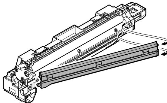
NOTE: All DV material must be removed before beginning step 2.
