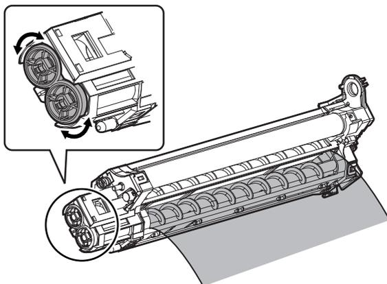
Since developer may remain in the front and the back sections, tilt the developing unit to remove all.
