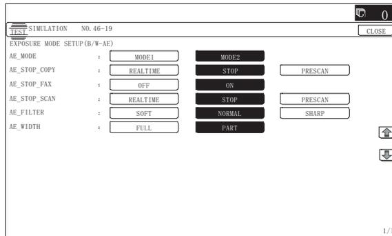
2) Set REALTIME, STOP or PRE-SCAN to adjustment item AE STOP COPY. For contents of each setting item, refer to below. Change the setting value of "AE WIDTH" item to "FULL" or "PART", in some cases.
