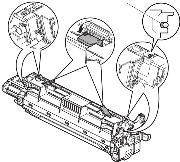
11) Shake the developing unit 5 - 6 times horizontally, and insert the developing unit straight and horizontally until it locks.
