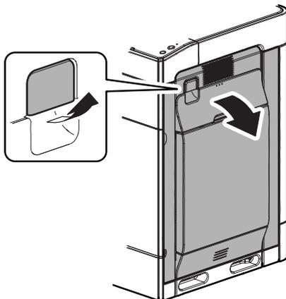
2) Pull the lever and remove the fusing unit.
