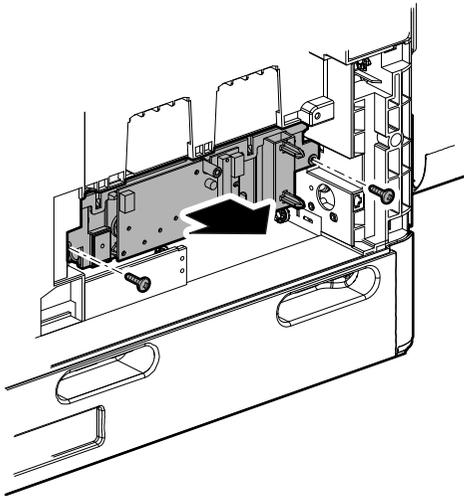
2) Remove the screw, and remove the polygon motor 1.
