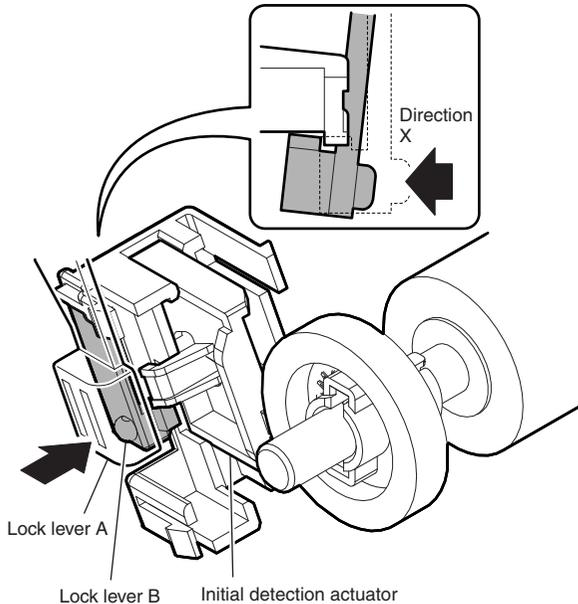
When the secondary transfer roller rotates, the secondary transfer unit initial detection actuator is shifted in the arrow direction Y by the drive gear.
