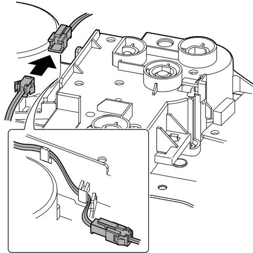
3) Remove the screw. Disengage the pawls (2 positions), and remove the belt separation frame unit.
