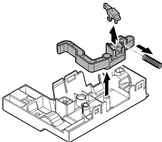
**D. Drum cartridge detection switch**
