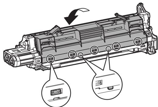
10) Lower the two levers and lock the cover.
