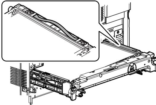
NOTE: When installing or removing the primary transfer unit, be careful not to touch the section marked with a red circle in the figure below. When opening the right door, be careful not to touch the exposed section of the transfer belt.
