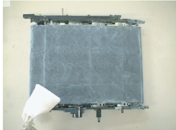
When replacing the transfer belt, perform the following procedures and observe the note in order to prevent reversion or meandering of the cleaning blade, or any trouble.
