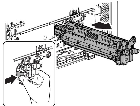
\* Tilt the developer unit so as not to disperse developer when removing the cover.
