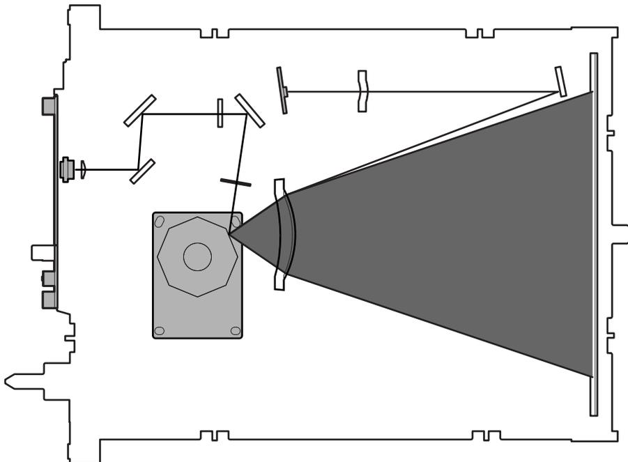
Laser beam generating section (SIDE)
