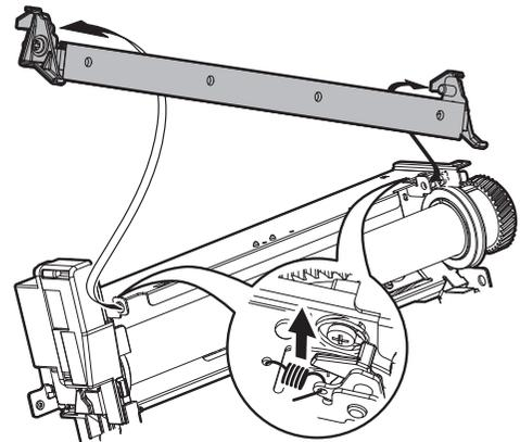
7) Remove the upper heat roller unit.
