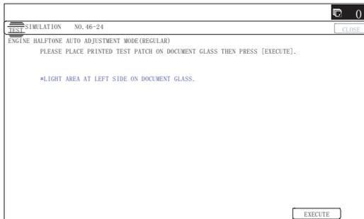
The copy adjustment is automatically executed to print the check patch image. Wait until the operation panel shown in procedure 5) is displayed.
