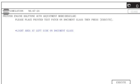
The printer density and gradation adjustment is automatically executed and prints the check patch image. Wait until the operation panel shown in the procedure 5) is displayed.
