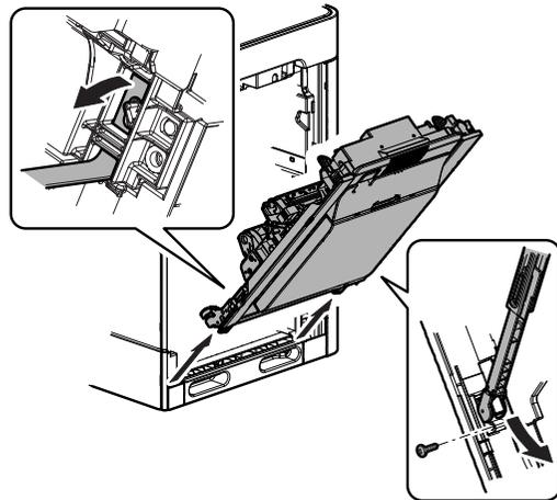
NOTE: When placing the right door, place so that the secondary transfer unit faces up.
