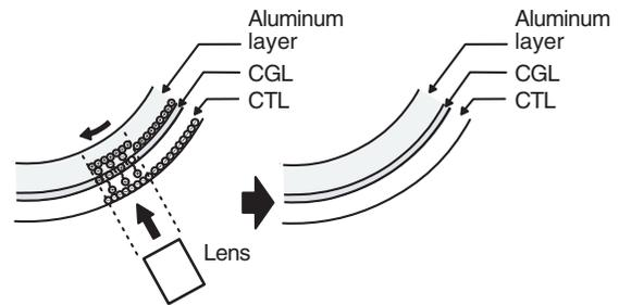
When the discharge lamp light is radiated to the discharge lens, the light is radiated through the lens to the OPC drum surface.
