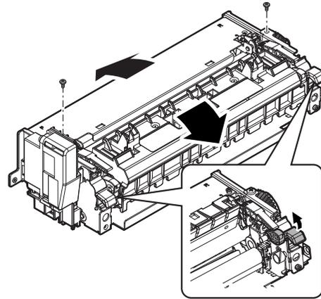
2) Remove the lower heat roller, and remove the lower heat roller bearing.
