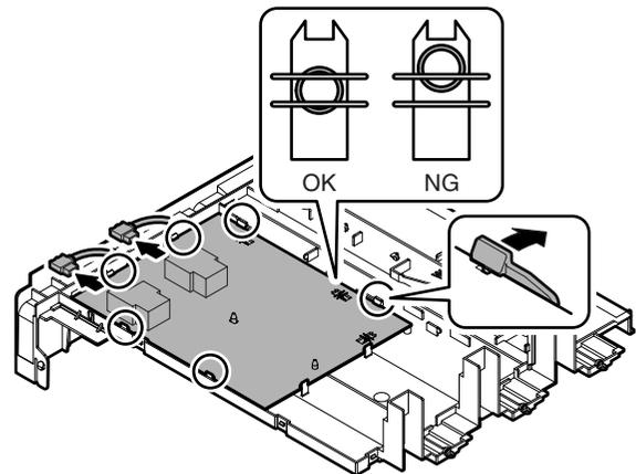
NOTE: When installing the PWB, check to confirm that there is no shift between the PWB terminal and the terminal on the high voltage PWB holder side.
