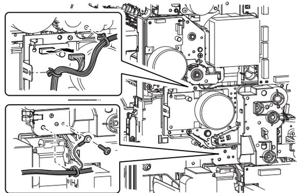
3) Remove the screw, and remove the main drive unit.
