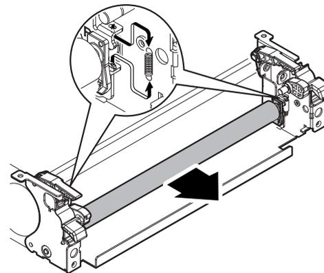
2) Remove the oil roller bearing and the cleaning roller.
