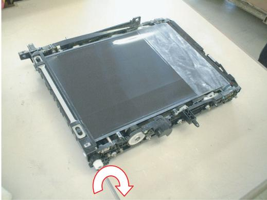
NOTE: \* The procedure to rotate the transfer belt must be executed on a flat surface. If not, the transfer belt may meander.
