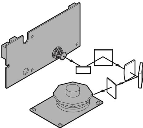
Laser beam generating section (Scanning image on paper)
