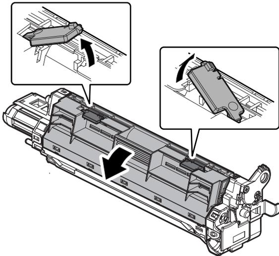
7) Turning the gear, take out the old developer.
