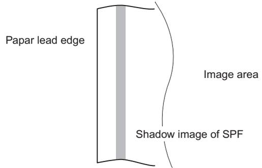
If the printed image at the leading edge of the copied image contains a shadow of the original table, then do the following steps.
