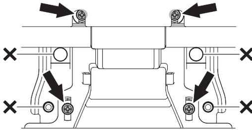
\* **Never loosen the screws marked with X.**
