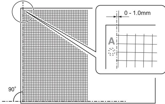
If the front surface copy image is as shown above and the back surface copy is not as shown above, go to the step 3) of "3. Skew adjustment (Back surface mode)."
