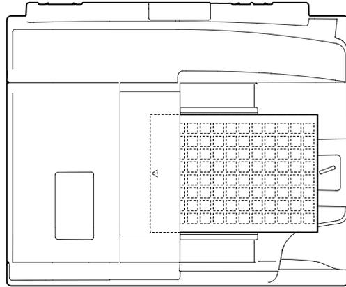
If the SIT chart is not available, execute SIM 63-5 to set the CCD gamma to the default. In this case, however, the adjustment accuracy is lower when compared with the adjustment method using the SIT chart.
