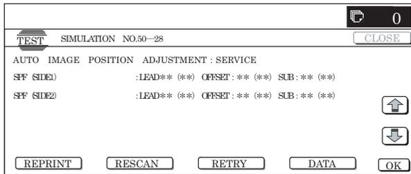
\* When [REPRINT] button is pressed, the display returns to the cassette select screen to allow self-print of the SPF adjustment pattern (front, back) again.
