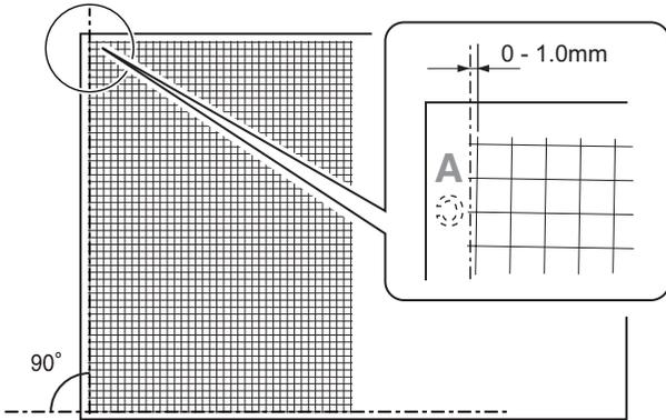
If the back surface copy image is as shown above and the front surface copy is not as shown above, go to the step 3) of "2. Skew adjustment (Front surface mode)."
