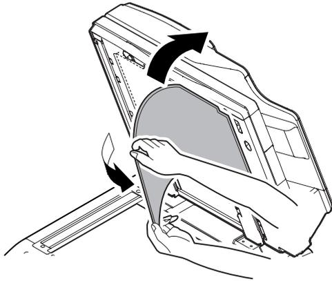
\* When assembling, place the OC mat on the document table to fit with the reference and close the DSPF unit.
