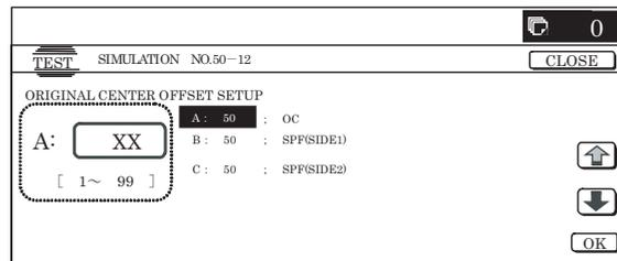
(UNIT: 0.1mm/STEP When the value is increased, the image is shifted to the front side.)
