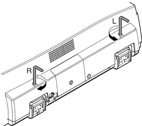
When the front frame side is higher (clearance B is more than 1mm): Turn the height adjustment screw R of the DSPF rear frame clockwise.
