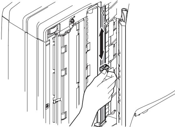
4) Remove the front cabinet. (Refer to "1. Exterior section - A. DSPF unit - (1) Front cabinet.")
