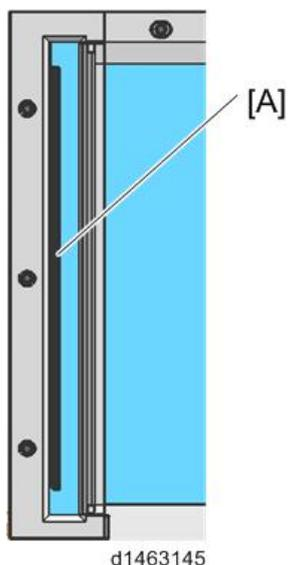
2. Wipe the exposure glass with alcohol, etc., so that no glue remains from the double-sided tape.
