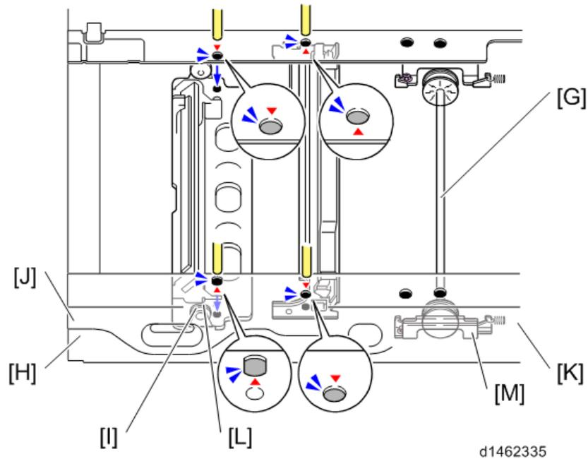
6. Set the pulley on the drive shaft [G] (tighten the screw temporarily).
