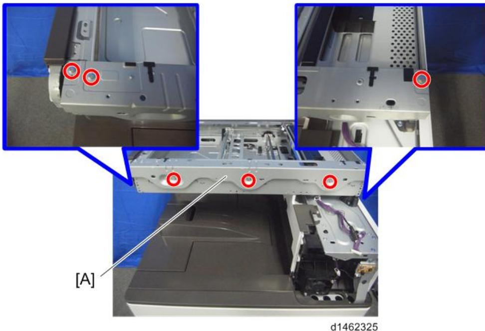
7. Move the 1st scanner carriage to the set position of the scanner fixing pin.
