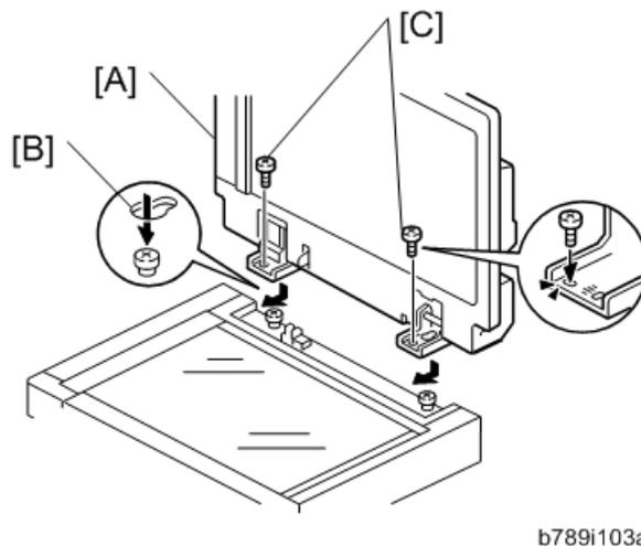
6. Align the rear left corner of the platen sheet [A] with the corner [B] on the exposure glass.
