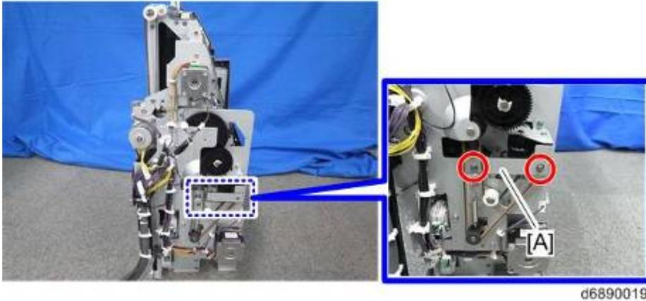
3. Remove the screw [A] of the belt holding bracket (⚙️×1)
