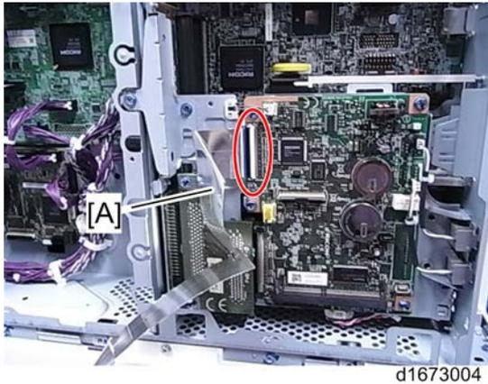
8. **Attach the FCU board removed in step 4 to the bracket. Then attach the flat cable to CN603 of the removed FCU board (⚙️ x 1).**
