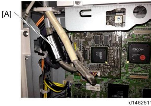
10. Attach the provided bracket [A] to the IPU board (🔩x1)
