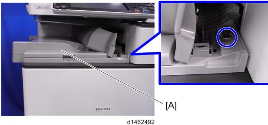
10. Attach the fixing plate [A] (🔩×1).
