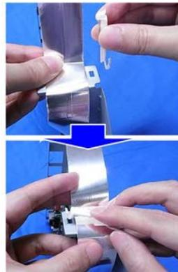
**7. Install the SG3 interface unit [A] (⚙️ x 3).**
