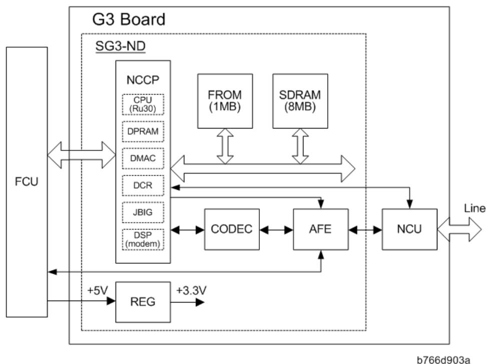
The SG3 board allows up to three simultaneous communications when used in combination with the FCU and optional G3 boards. The NCU is on the same board as the common SG-3 board. This makes the total board structure smaller. But, the specifications of the SG3 board do not change.
