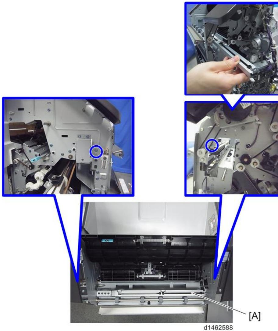
11. Insert and attach the registration sensor unit [A] from the rear (⚙️x2).
