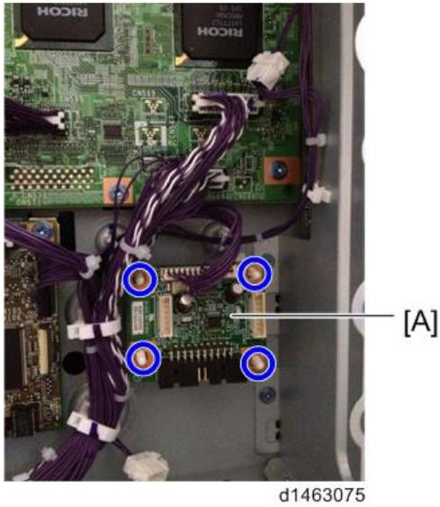
3. Connect the harness of the MFP to the upper connector (white/13 pin) [A].
