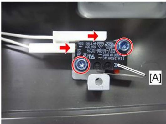
4. Pick-up roller HP sensor [A] along with the bracket (🔧×1, 📌×1, 📌×1)
