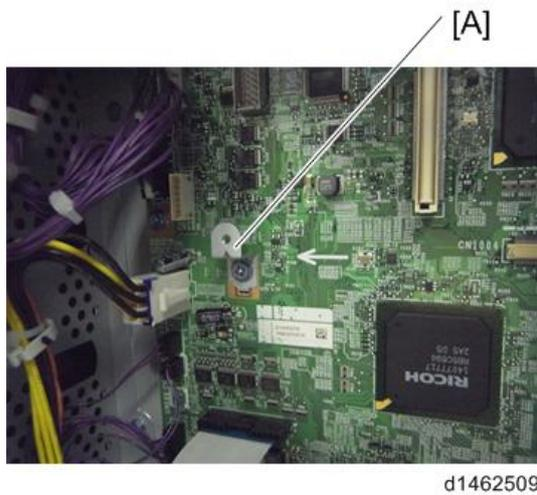
11. Attach the IPU sub board [A], and insert the connector of the scanner cable (🔩x3)
