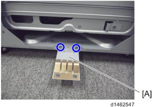
9. Attach the connecting brackets [A], [B] to the machine (⚙️×4).
