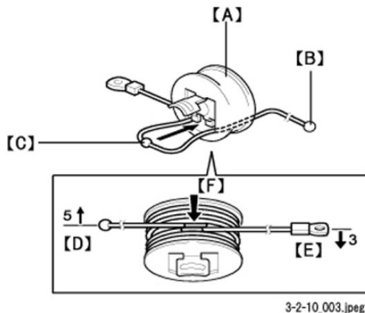
1. Pull the scanner wire ball end [B] to the pulley [A] from the left side of the pulley as shown in the diagram.
