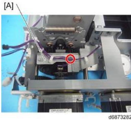
3. Center-folding cam HP sensor [A] (📺×1)
