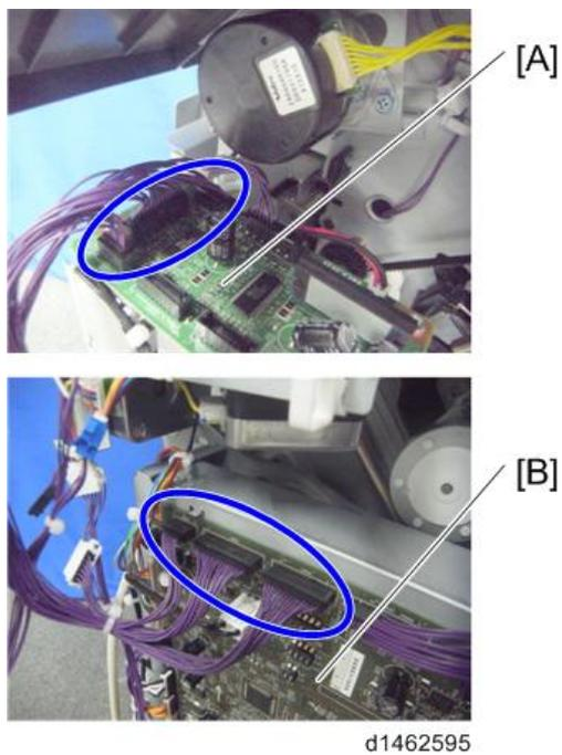
17. Remove the harness [A] from the clamp [B], and connect it to the punch unit board [C] (☐x1).
