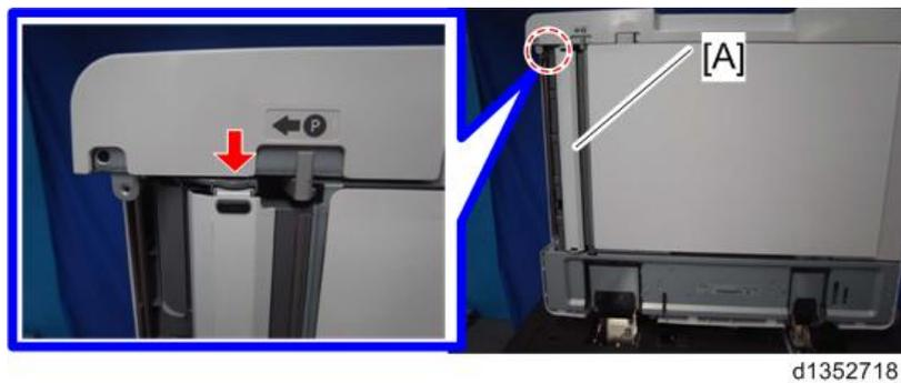
3. Original registration sensor [A] along with the bracket (🔩×1, 📌×1)
