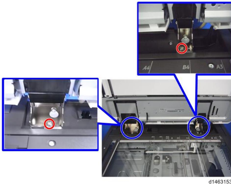
9. While holding the left and right sides of the ADF, lift up to remove it.
