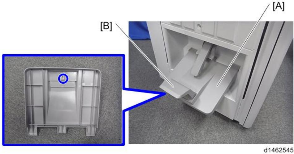
8. Attach the relay guide plate [A] (⚙️×2).
