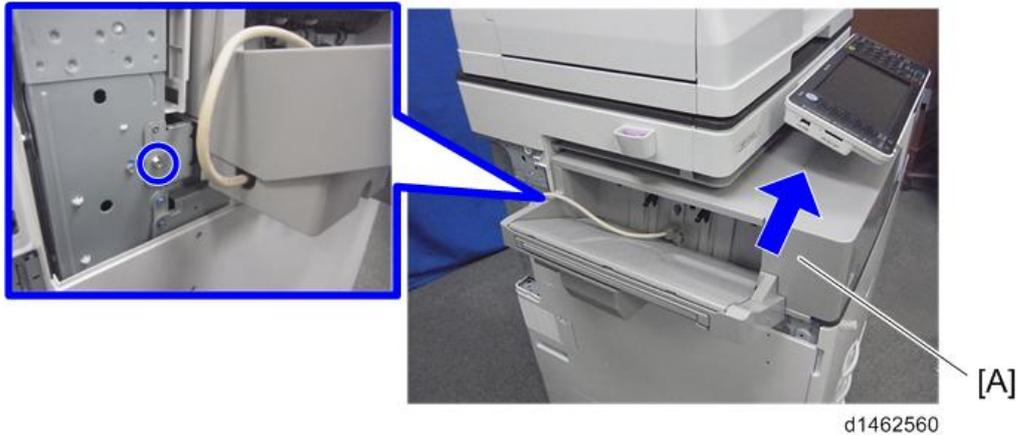
12. Attach the components [A] and [B] to the finisher (⚙️×2).
