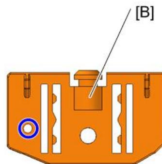
4. Replace the contactless guide plate (rear) [A] with the contact guide plate (rear) [B].
