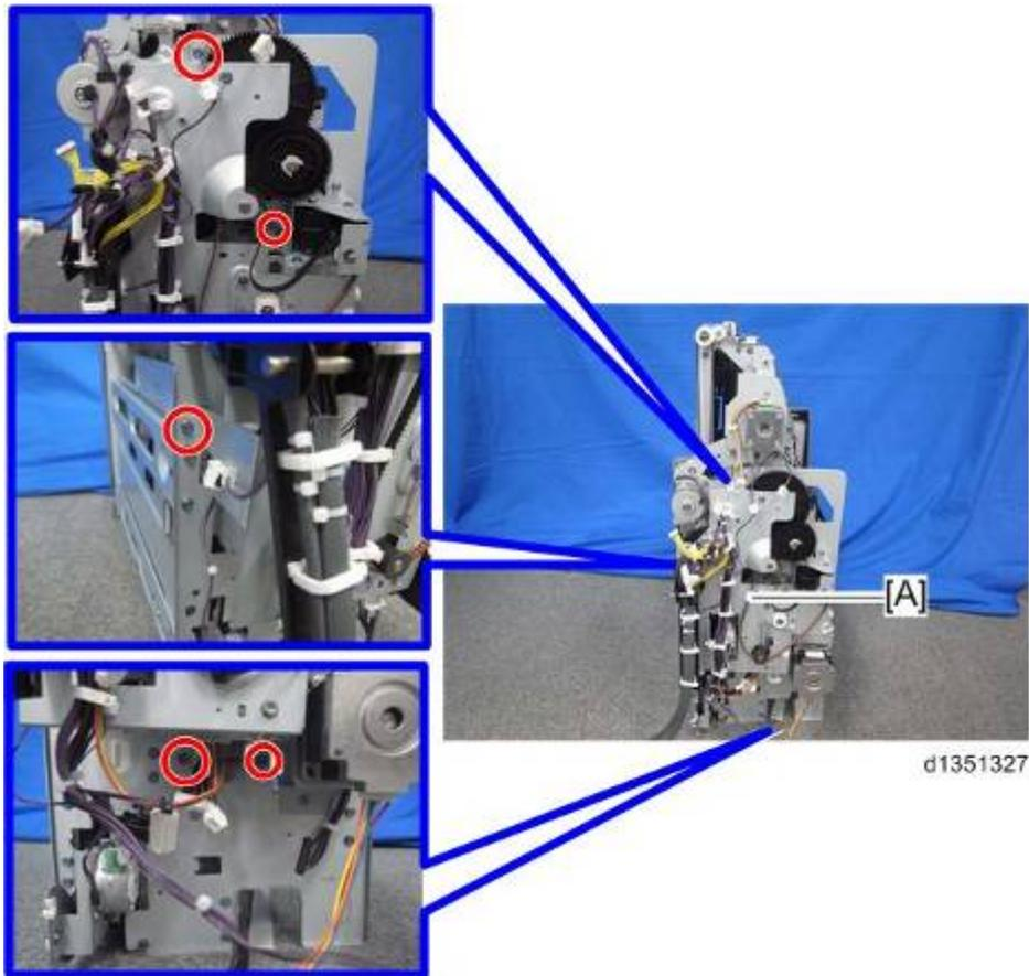
9. Remove the spring [B] from the press folding motor bracket [A] (⚙️×1, spring×1)
