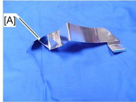
**10. Attach the flat cable [A] to the bracket of the SG3 interface unit with the clamp [B].**
