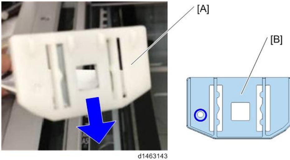
5. Attach the document reader guide plate. Be careful not to scratch the sheet [A].
