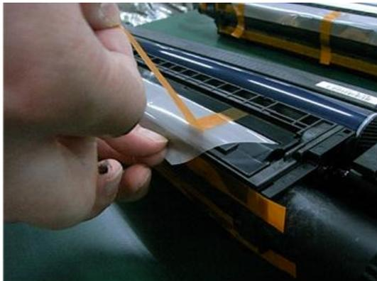
11. Remove the preset seal [A] in the direction of the blue arrow.
