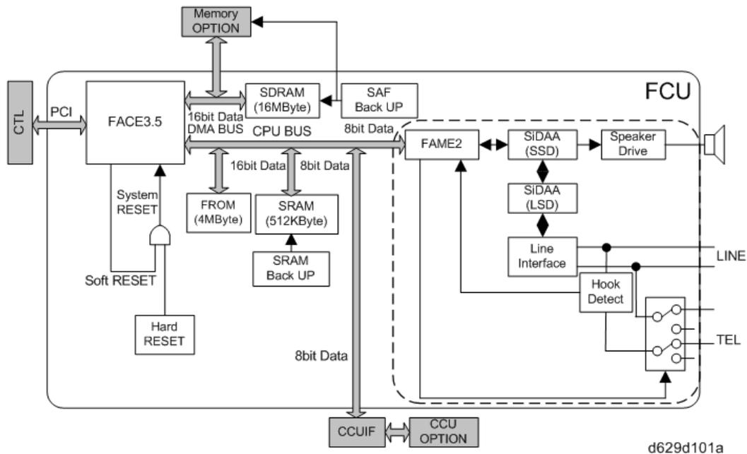
The FCU (Facsimile Control Unit) controls fax communications, the video interface to the base copier's engine, and all the fax options.
