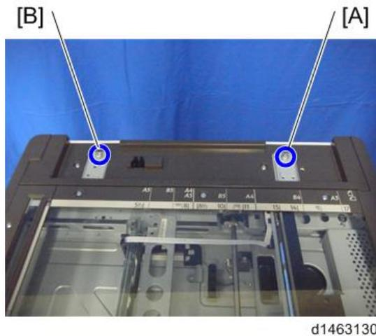
3. Mount the ARDF [A] by aligning the screw keyholes [B] of the ARDF support plate over the stud screws.
