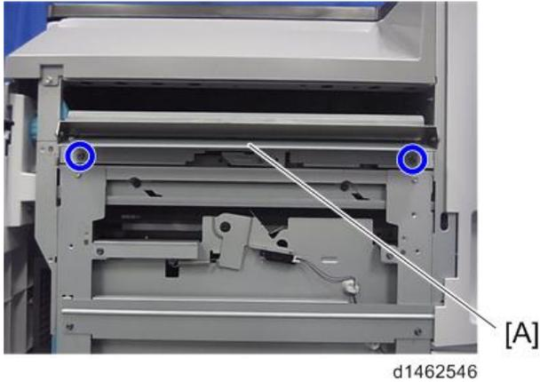
8. Attach the ground plate bracket [A] (⚙️×2).
