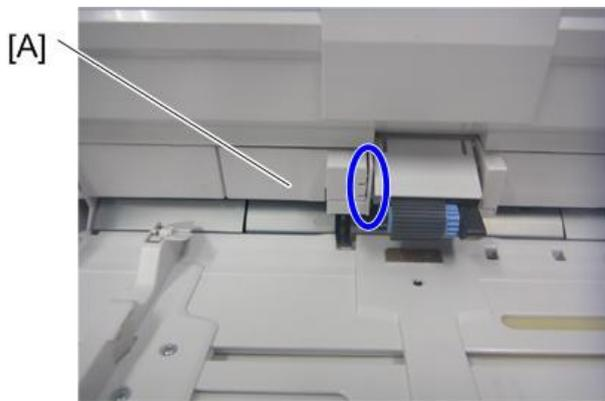
3. By-pass paper end sensor unit [A] (⚙️x1, 🔧x1)
