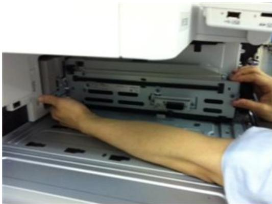
8. When installing the punch unit in a finisher that is already installed, remove the relay guide plate [A] (2x).
