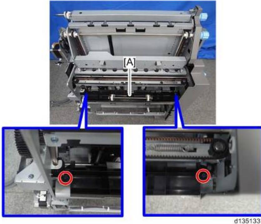
3. Open the bracket [A] of the flat fold roller.
