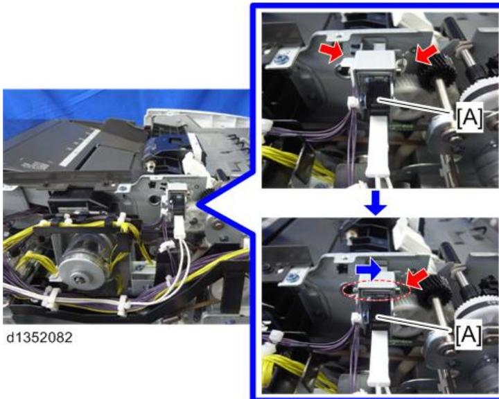
3. ADF feed cover interlock switch [A] (🔧×2, 📌×2)
