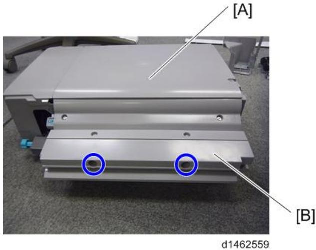
22. Slide the finisher [A] along the rail of the bottom plate from the left-hand side of the machine to attach it (⚙️x1).
