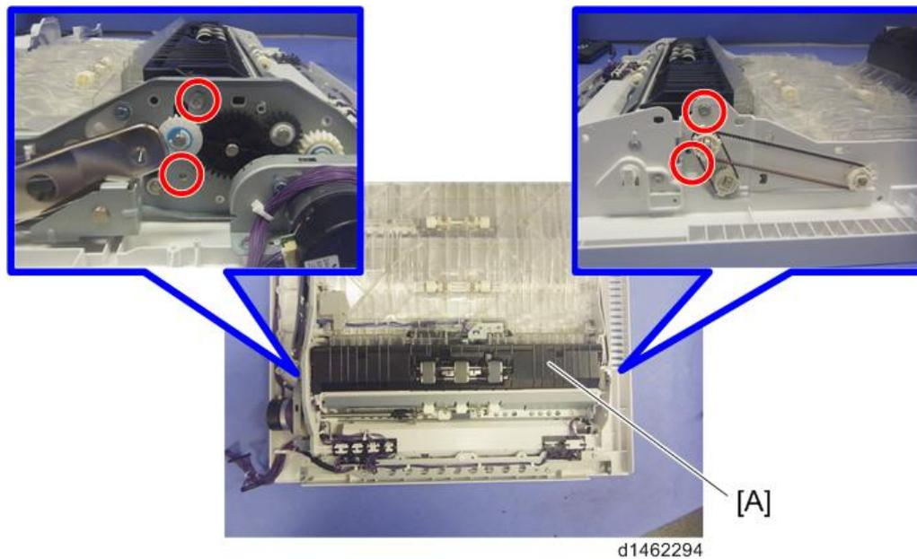
5. Double feed sensor unit [A] (🔩x2)
