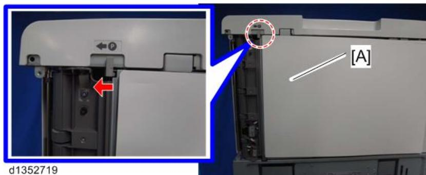
4. Remove the original exit sensor [B], which is mounted on the upper guide [A] (🔩×6)
