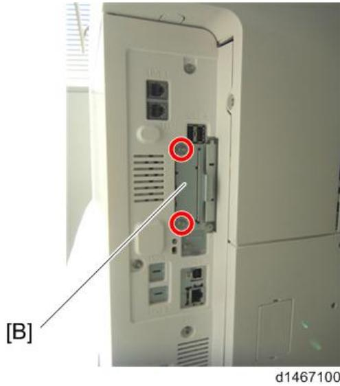
2. Set the File Format Converter in an I/F slot (🔑x2)
