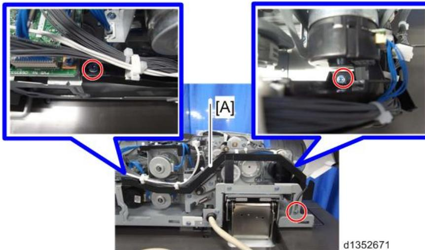
3. ADF pick-up roller lift motor [A] (🔧×2, 📏×1, timing belt×1)
