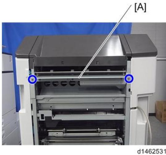
9. Attach the ground plate bracket [A] (⚙️×2).
