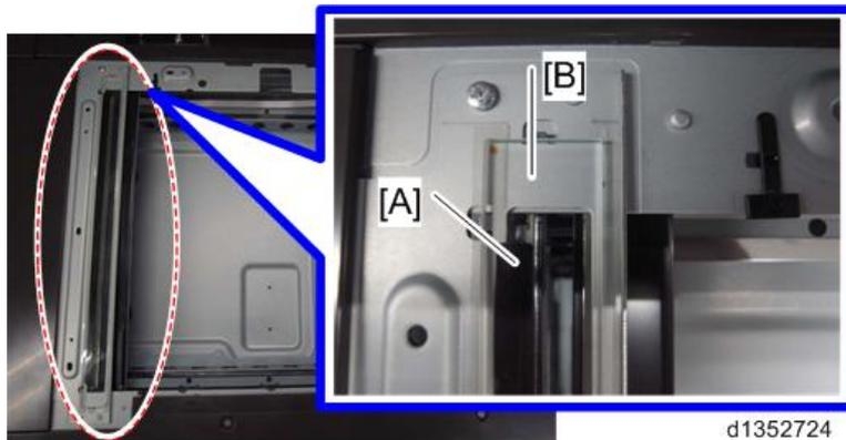
3. Wipe the exposure glass with alcohol, etc., so that no glue remains from the double-sided tape.
