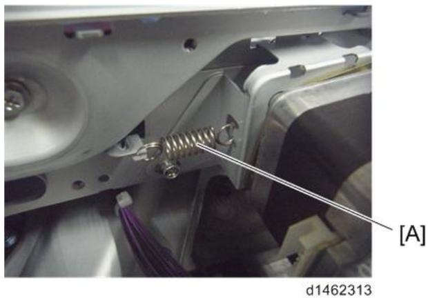
5. Scanner motor unit [A] (⚙️x2, 📦x1)
