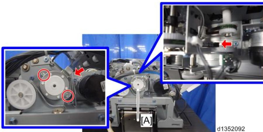
4. ADF transport motor [A] along with the bracket (🔧×2, 📏×1, timing belt×1)
