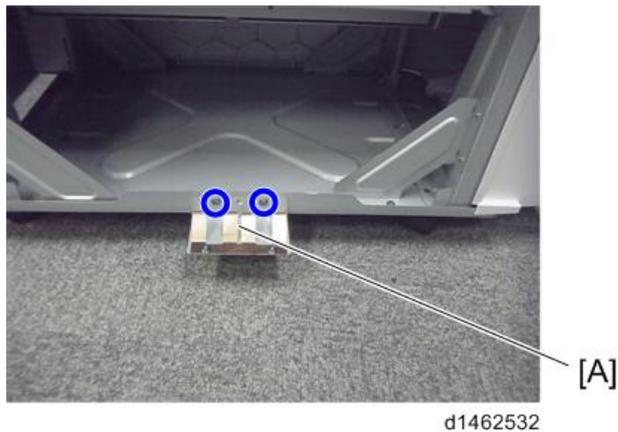
10. Attach the connecting brackets [A], [B] to the machine (⚙️×4).
