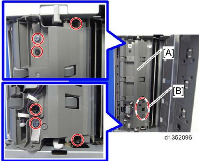
5. Remove the original exit sensor [B] from the upper guide [A] (🔧×1, 🛠️×1)
