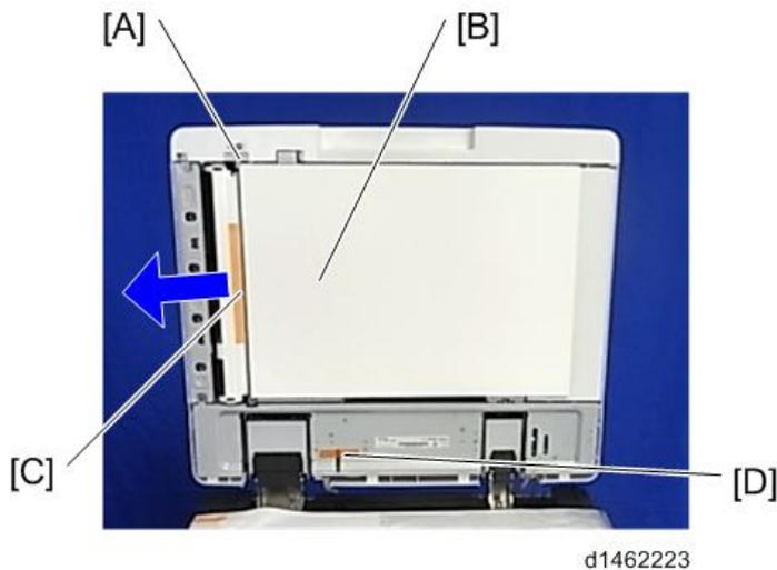
7. Remove the filament tape [D].
