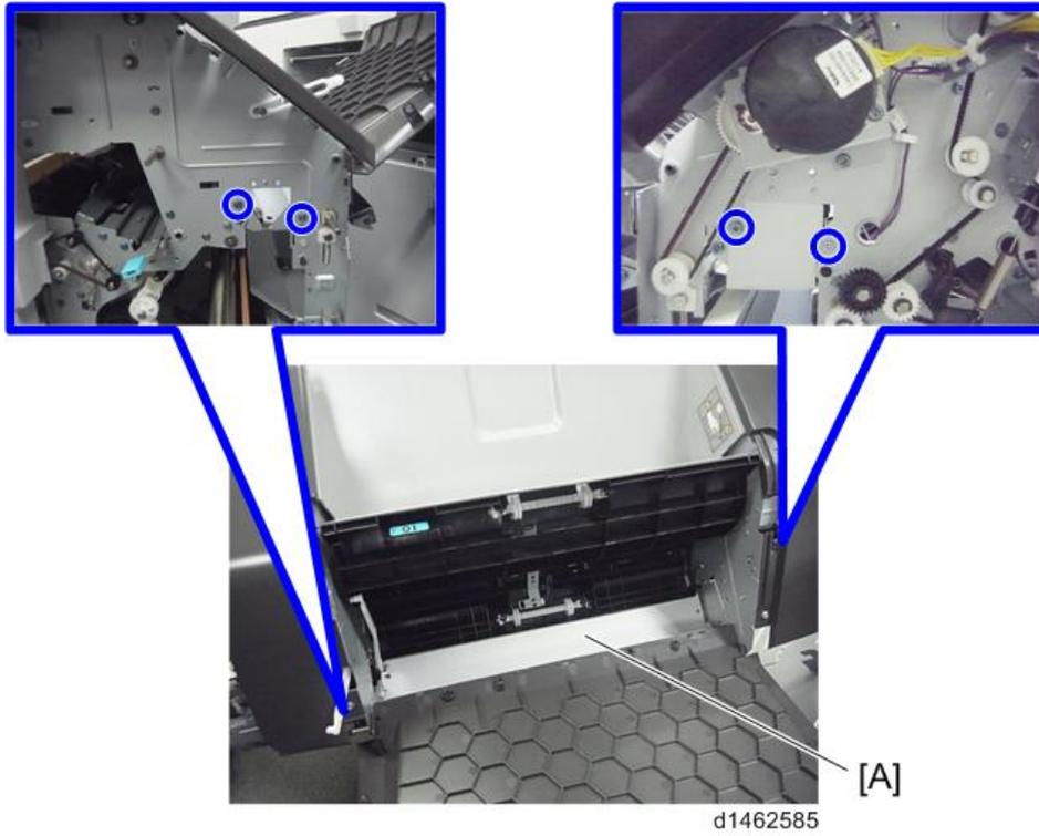
8. Insert and attach the hopper guide plate [A] from the front (⌀×4).
