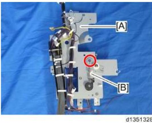
10. Remove the press folding motor [A] (⚙️×2, ⚙️×1)
