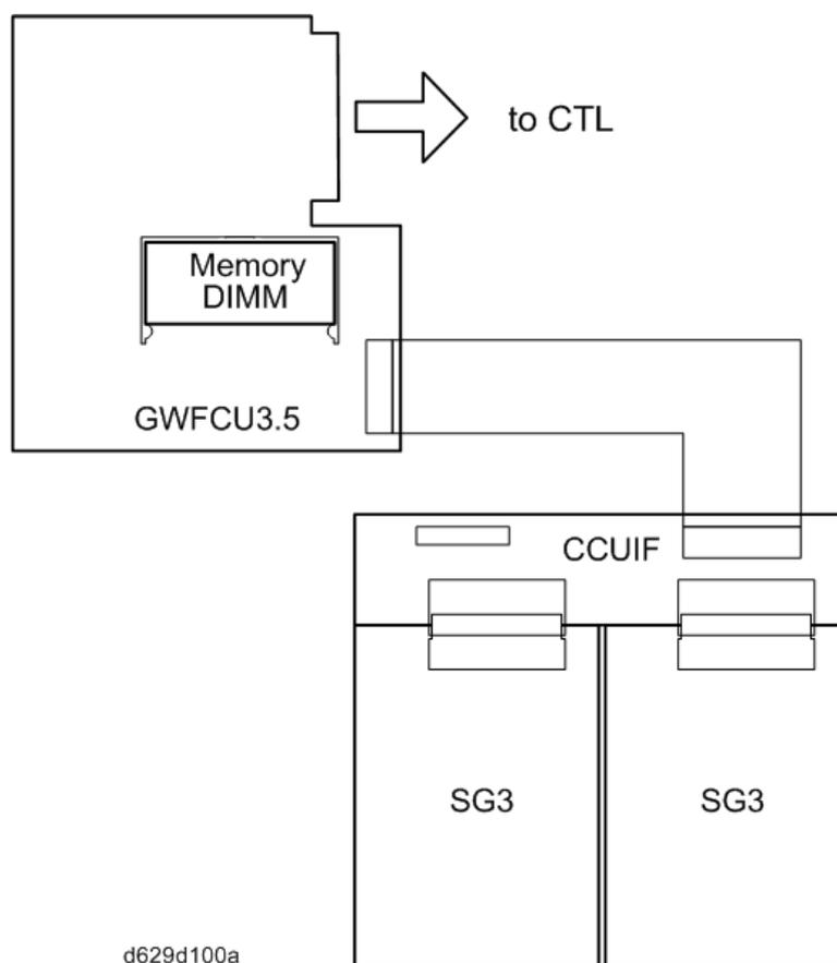
The FCU controls all the fax communications and fax features, in cooperation with the controller board. Also, the FCU contains the ROM, SRAM and NCU circuits.
