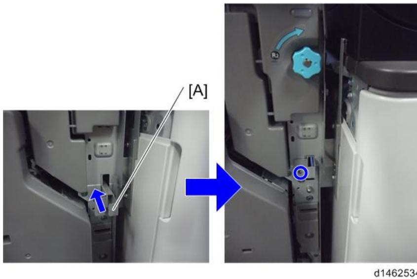
12. Attach the arm of the anti-tip component [A] (1x1). (Finisher SR3140 only)
