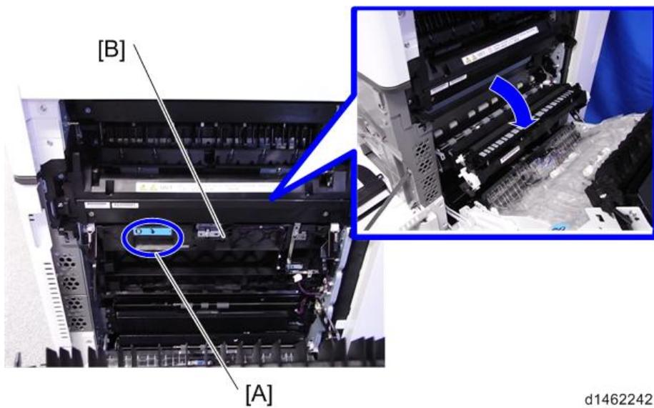
5. Release the ITB lock lever [A] and ITB contact lever [B].
