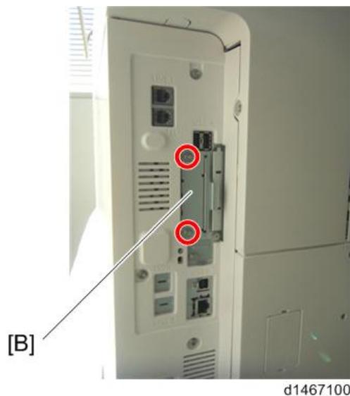
2. Attach the extended wireless LAN board to a slot (🔩x2)
