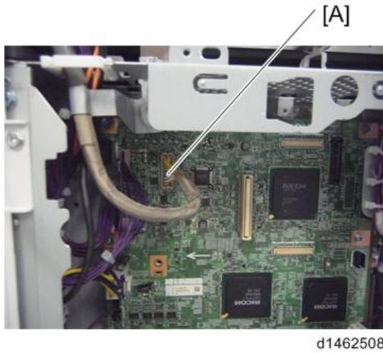
9. Attach the provided ferrite core [A] to the scanner cable.
