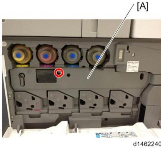
3. Release the lock [A] and open the right cover [B].
