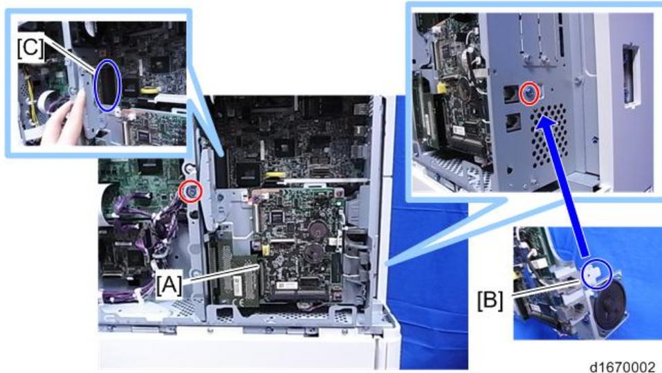
4. Replace the installed FCU board [A] with a new FCU board (⚙️ x 4, 📠 x 3).
