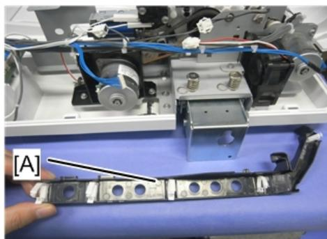
4. Feed motor with bracket [A] (🔗 x 2, spring [B] x 1)
