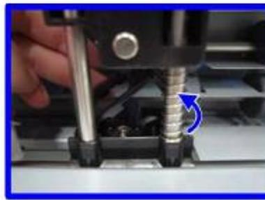
4. Adjust the position of the flat fold lower roller [A] to adjust the difference in alignment between the upper and lower rollers of the flat fold booklet unit.
