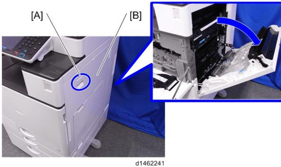
4. Pull the handle [A] and open the paper transfer unit [B].
