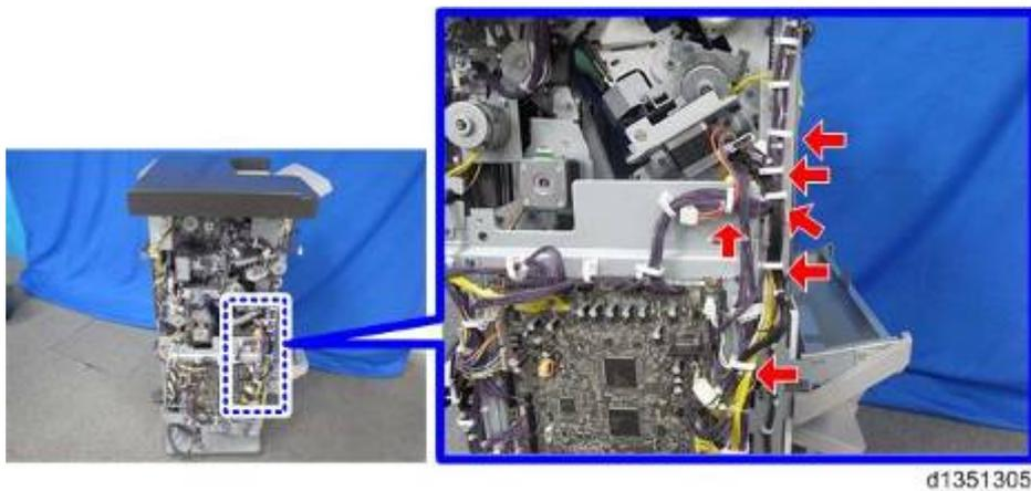
12. Remove the ground wire [A] of the main board (🔧×1)
