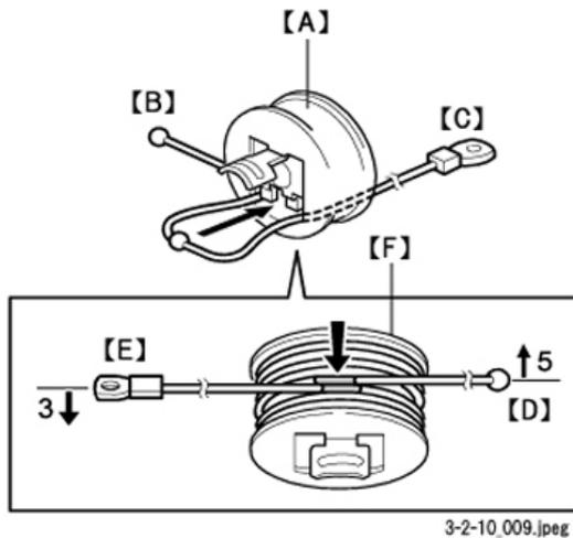
1. Pull the scanner wire ball end [B] to the pulley [A] from the right side of the pulley as shown in the diagram.
