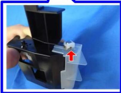
4. Lift the left and right sides of the feed belt holder [A], then remove it.
