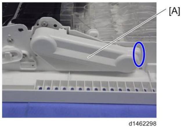
4. Remove two tabs, and remove the vertical transport guide plate [A] (4).
