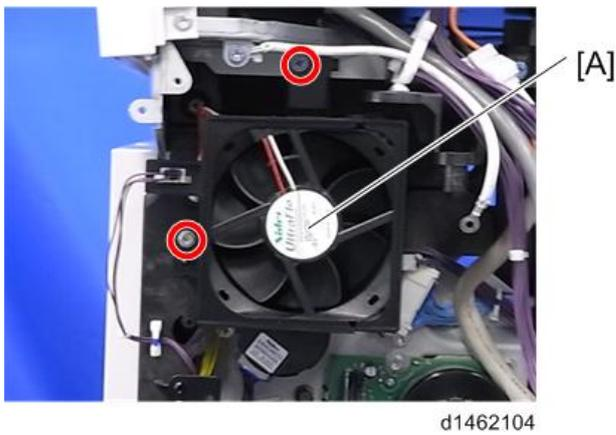
3. Fusing exhaust heat fan [A]
