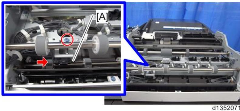
4. Remove the original width sensor guide plate [A] (🔩×2), then remove the original width sensors (📏×5) [B] (hook×1 each)
