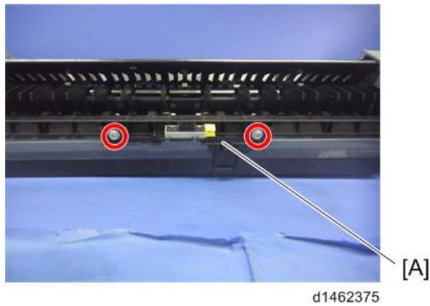
3. Fusing exit sensor [A]
