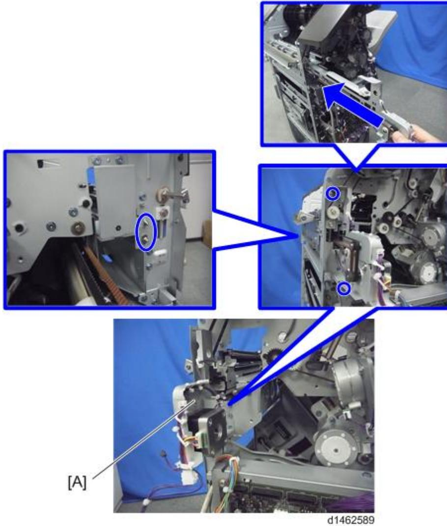
12. Connect the harness [A] of the hopper guide plate to the relay connector [B] of the registration sensor unit.
