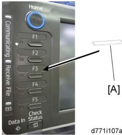
12. Attach the serial number decal under the copier serial number decal on the rear cover of the machine.
