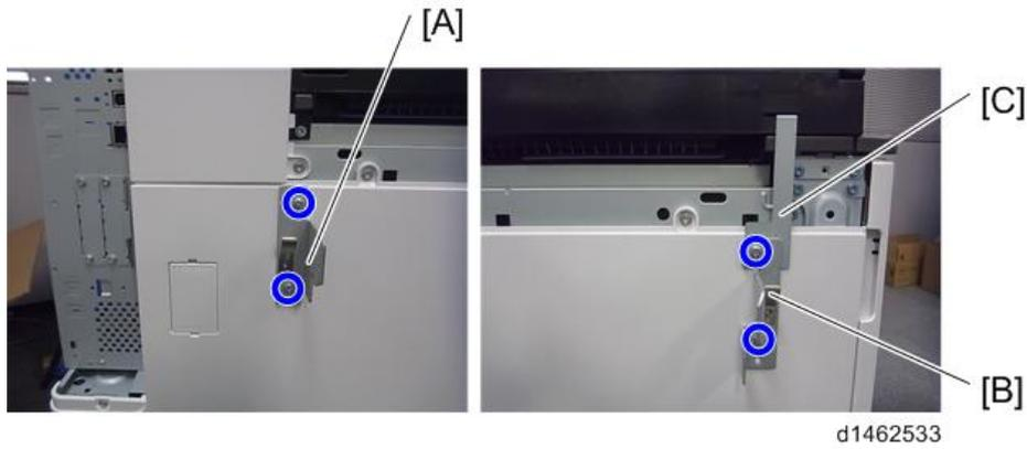
11. Connect the finisher to the machine with the connection lever [A] (1x1).
