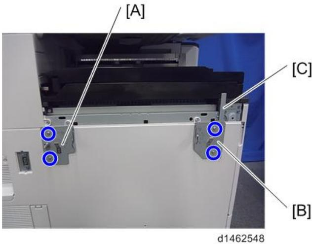
10. Connect the finisher to the machine with the connection lever [A] (⚙️×1).
