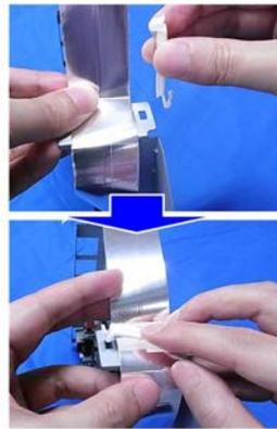
**11. Install the SG3 interface unit [A] (⚙ x 3).**
