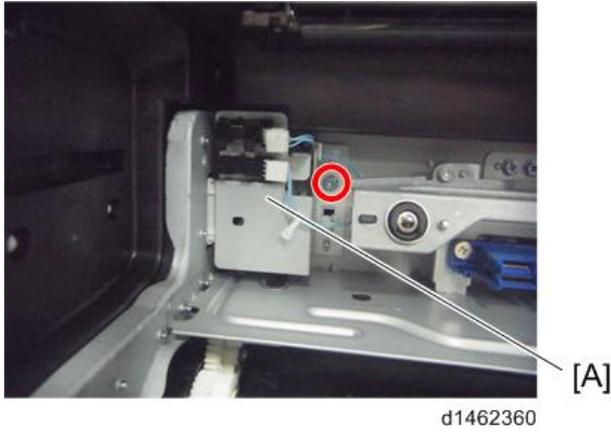
3. Fusing shield position sensor (upper) [A], Fusing shield position sensor (lower) [B]
