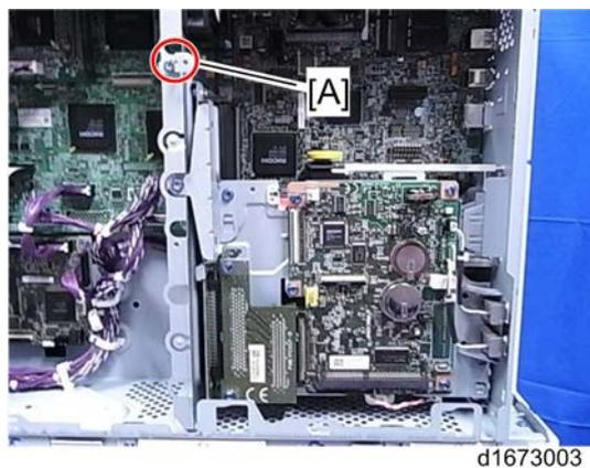
7. Attach the flat cable [A] to CN603 of the new fax unit.
