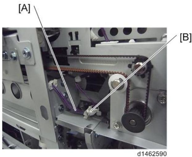
13. Insert and attach the punch unit [A] from the rear (⚙️x2).
