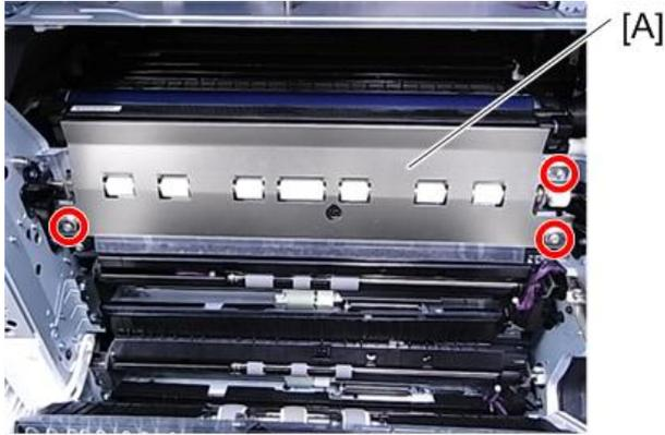
4. Remove the registration sensor from the stay gap using a slotted screwdriver (🔧×1)
