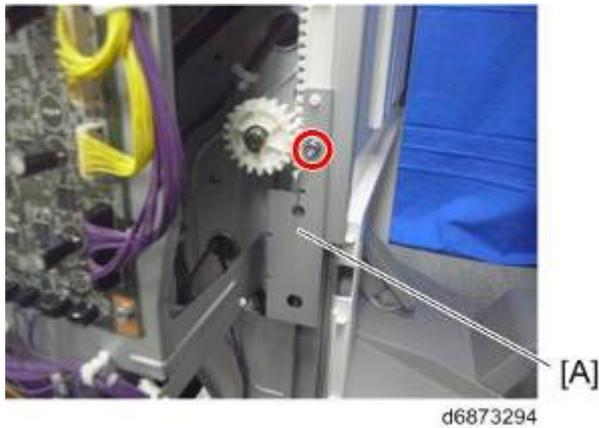
3. Control board bracket [A] (🔧×5, 📏×21, 📏×17, ground plate×1)
