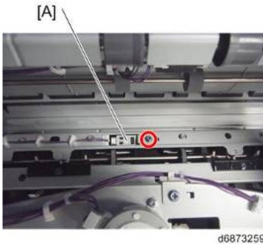
3. Intermediate transport (left) paper surface sensor [A]
