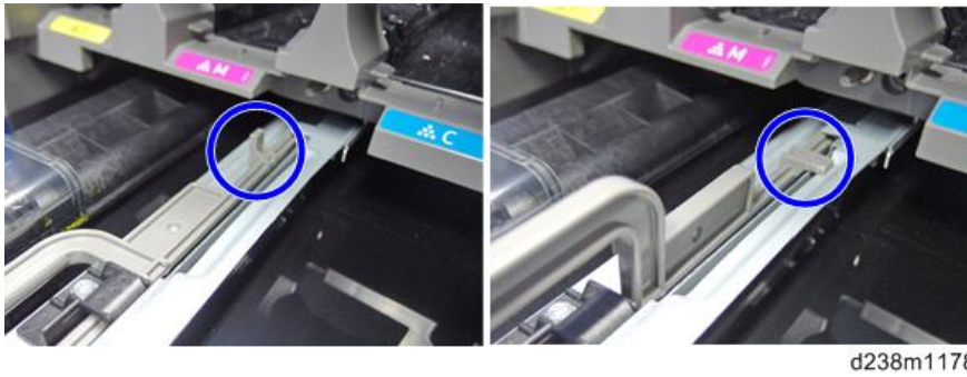
Locking mechanism by handle
