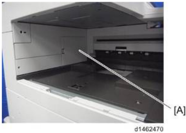
12. Paper output lower cover [A] (🔩 x3).
