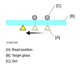
Dirt/soiling is detected when a document passes through, so the alert will not disappear until reading of the next document begins, even after target glass cleaning is performed. If dirt/soiling is detected not on the target glass but on the background guide plate, the alert will not disappear even if the glass is wiped.
