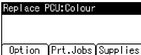
When the following messages appear on the display, the photo conductor unit should be replaced soon. Prepare a new photo conductor unit.
