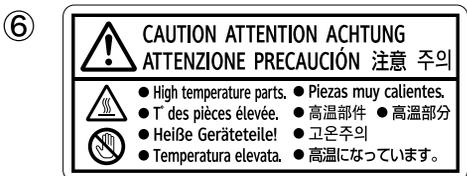
⑥ The inside of the machine could be very hot. Do not touch the parts which a label is put on. Otherwise, an injury might occur.
