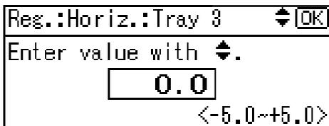
Increase the value to shift the print area in the direction indicated by the “+” symbol in the diagram below. Decrease to shift the print area in the direction indicated by the “-” symbol.
