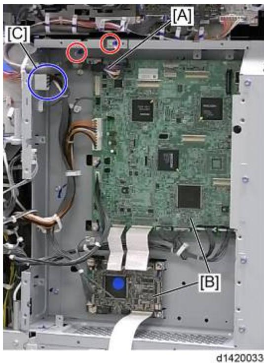
7. Disconnect the scanner interface cable [A] (ground cable)
