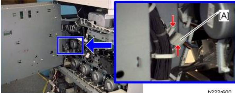
5. Disconnect the connector [A] (🔌 x 1, 🗑️ x 1)
