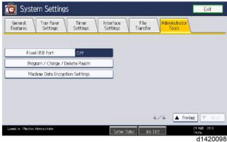
4. Press the [Machine Data Encryption Settings].
