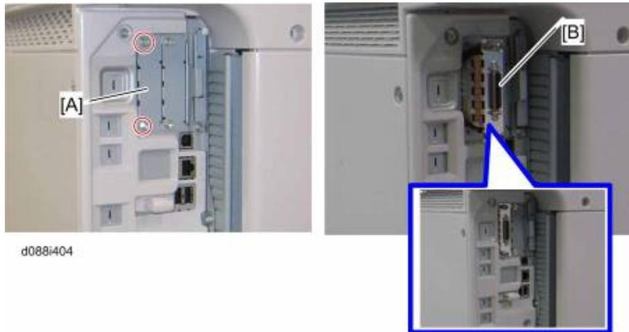
1. Remove the slot A cover [A] (
