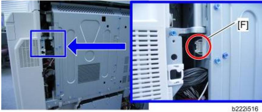
6. Connect the harness to the connector [F] inside the machine.
