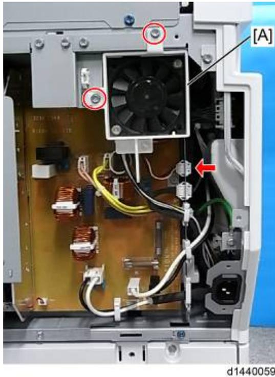
2. Tube cooling fan bracket [A] ( x 2, x 1)
