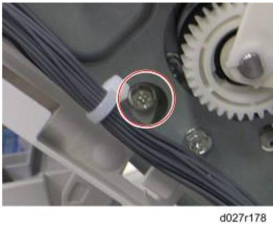
8. Remove the screw at the rear side.
