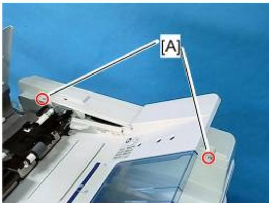
4. Remove two screws [A] on the ADF rear cover [C].
