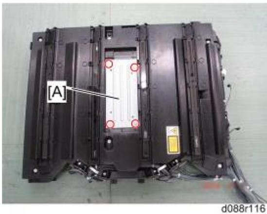
2. Polygon mirror motor cover [A] of the laser optics housing unit (
