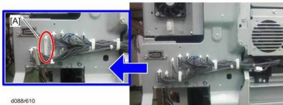
3. Disconnect the harness [A] of the skew correction motor.
