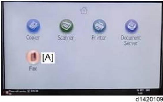
If the fax icon is not displayed (as shown below), the FCU should be replaced. Refer to the Fax service manual for the FCU replacement procedure.
