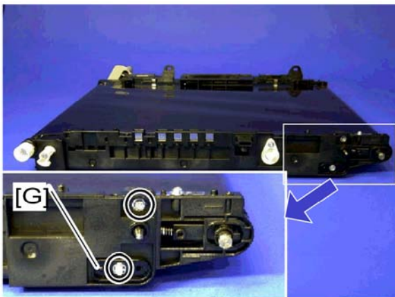
9. Remove the two screws and then rear hold bracket [G] (as seen from the rear).
