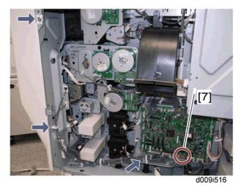
6. Connect the harness to CN211 [7] on the IOB ( ${\textcircled{}} x$  3).
