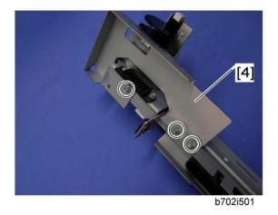
4. Remove the bracket [4] from the punch unit ( $\mathscr{F} \times 3$ ).
