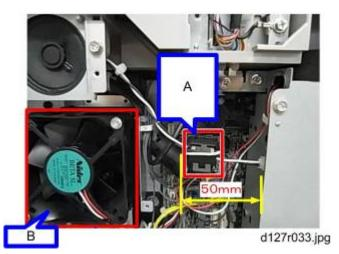
7. Attach the ferrite core [A] on the speaker harness within 50mm from the end of the controller board. This prevents the harness from being involved in the fan [B].
