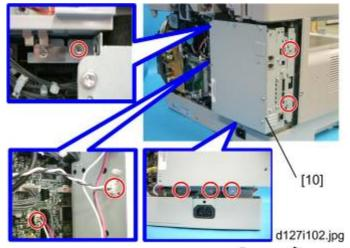
10. Remove the controller box [10] ( x 2, x 6).
