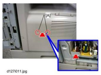
Make two holes [A] through which the screws fasten the handset bracket to the main machine.
