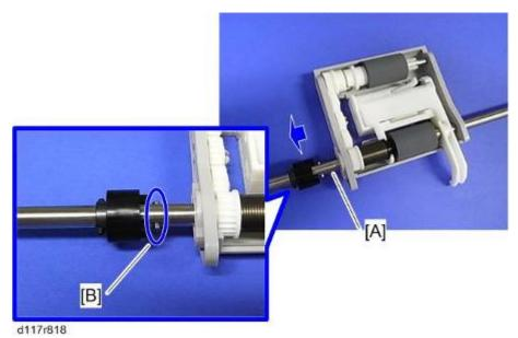
3. Slide the shaft [A], and then remove the pin [B].
