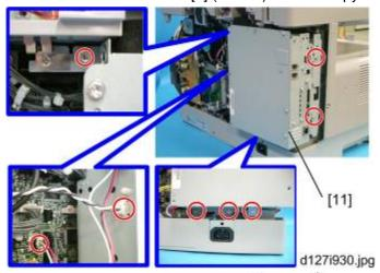
11. Remove the controller box [11] ( x 2, F x 6).
