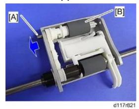
3. Slide the shaft [A], and then remove the pick-up roller [B].
