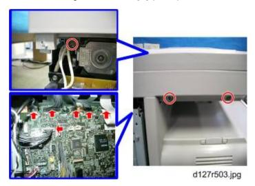
3. Remove the screws and the harnesses showed above for detaching the scanner unit.
