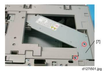
8. Attach the harness cover [7] ( x 2, Washer x 2, Spring Washer x 2).
