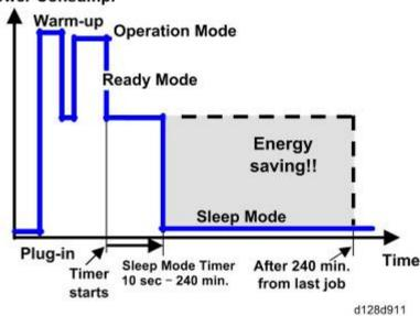
The area shaded grey in this diagram represents the amount of energy that is saved when the timers are at the default settings. If the timers are changed, then the energy saved will be different. For example, if the timer is set to 240 min., the grey area will disappear, and no energy is saved before 240 min. expires.
