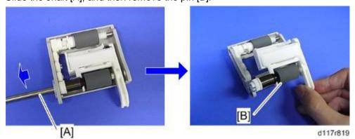
4. Slide the shaft [A], and then remove the feed roller [B].
