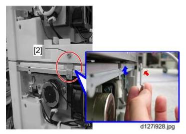
2. Attach the joint bracket (Rear) [2] as shown. ( 🔊 x 2)
