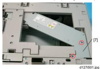
8. Attach the harness cover [7]. ( x 2, Washer x 2, Spring Washer x 2)
