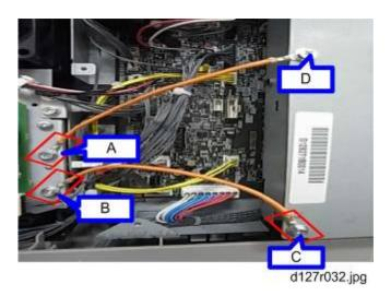
Attach the grounding wire as shown.
