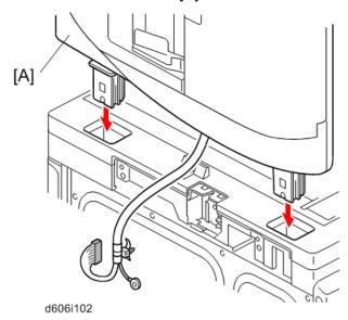
6. Remove the ARDF [A] from the copier as shown.
