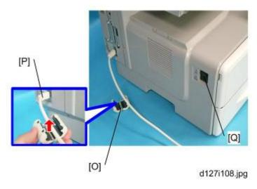
21. Attach the ferrite core [O] to the end of the network cable [P] when connecting the cable.
