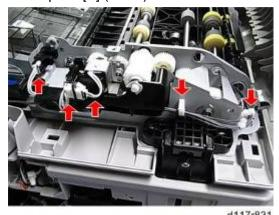
4. Release the clamps and disconnect the connectors (🗗 x 3, 🚔 x 2).
