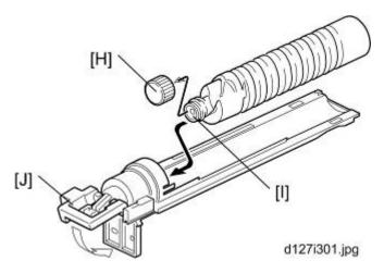
7. Remove the outer cap [H].
