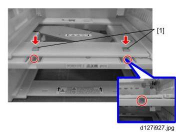
1. Attach the joint bracket (Front) [1] as shown. ( \*\mathbb{F} x 2)
