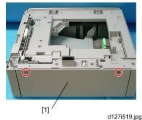
2. Remove the rear cover [1] from the paper tray unit ( \*\bar{p} x 2).
