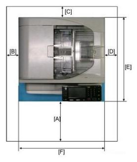
A (Front) 750 mm (29.6") 100 mm (3.9") B (Left) 100 mm (3.9") C (Rear) 100 mm (3.9") D (Right) E Depth 450 mm (17.7") F Width 476 mm (18.7")
