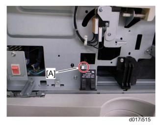
4. Connect the harness [A] to the mechanical counter.
