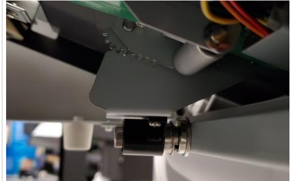
Magnetic catch and lock parts bar latched
