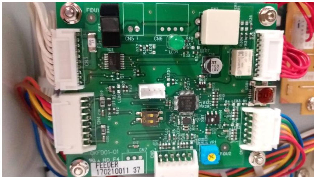
New Style Controller Bd., for all production envelope feeders No Amber LEDs on it.
