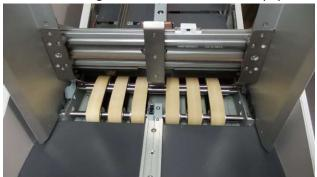
b. Scrape the belts back and forth vigorously. It is easiest when pulled in the direction of the user.
