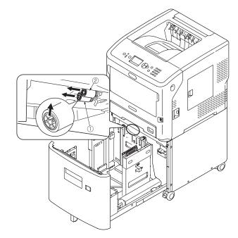
(3) Put the new roller (with gear)  $\bigcirc$  to the shaft.
