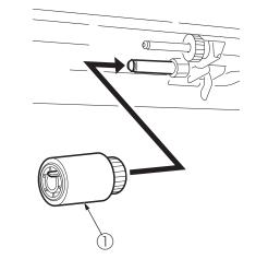
(4) Put the new roller (with gear) 2 to the shaft.
