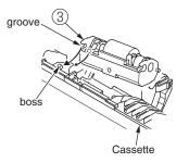
(11) Assemble the Retard Roller 3 to push the Retard Roller 3 to Cassette, and push up front side.
