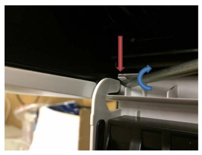
6. The hinge locking tab in the open position
