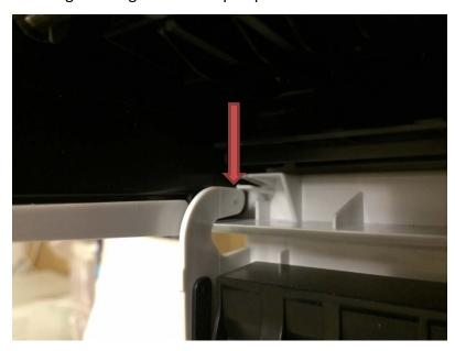
7. Push on the outside of the ADF Top Cover hinge to move the hinge pivot pin out of its mounting hole.
