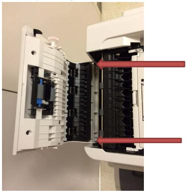
4. Find the ADF Top Cover hinge locking tab.
