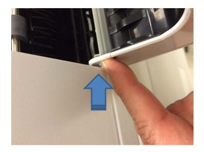
8. Hinge pivot pin out of position.
