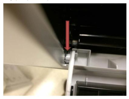
9. Repeat steps 5, 6, and 7 for the other hinge and remove the ADF Top Cover
