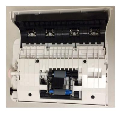
11. Loosen the 4 mounting screws (a) of the "Top Guide Assy."
