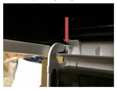
5. Use a flat blade screw driver to gently move the tab to the unlock position
