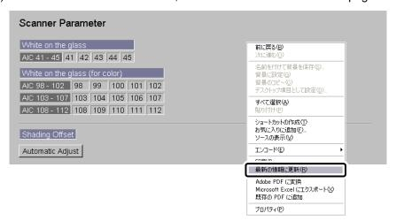
(5) Check to confirm that the **Shading Offset** calibration value has been updated.
