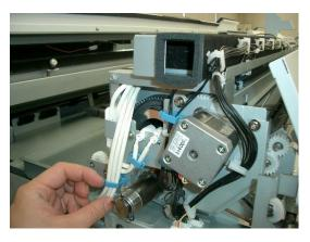
**9.** Loosen the one screw of the plate securing the connector, then remove the plate.
