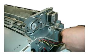
(b) Move the loosened screw to the right side of the guide and tighten it temporarily.
