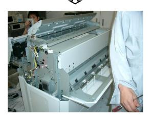
**6.** Loosen the two screws securing the glass on the left side of the scanner cover shown in the photo.
