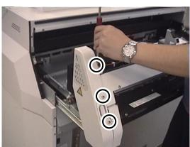
(c) Remove the COVER-FUSER-L with three screws.
