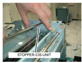
**5.** After installing the front-side guide plate (GUIDE-FRONT-SC) on its position, secure the four screws while applying a light amount of pressure to the CIS UNIT.
