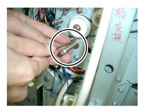
**11.** On the right side of the Printer, remove the E-ring on the other side of the shaft, and remove the bearing.
