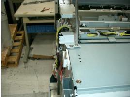
3. Remove the plate with one screw from the right side of the Printer at the location shown in the photo.
