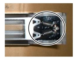
**2.** With a set of tweezers, remove the plastic parts both on the right and the left shown in the photo.
