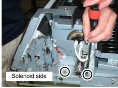
Type B: Fuser unit fixed with four screws mounted from lower side.
