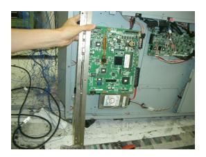
**6.** Remove the three screws securing ARC and COVER-SIDE-L.
