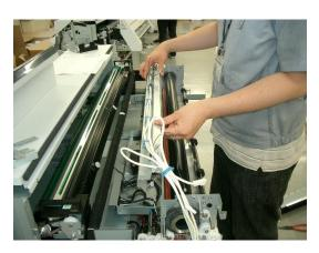
**8.** Remove the HR-CAP on the left edge of ROLLER HEAT.
