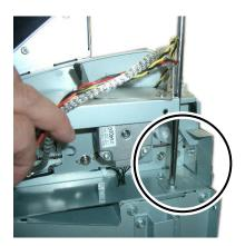
**4.** Remove the two screws of the plate securing ROTARY-DAMPER-R, shown in the photo.
