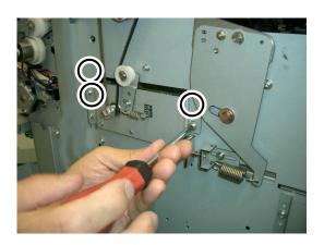
**6.** Remove the timing belt and pull out the PM01 slightly.
