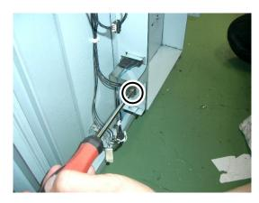
**5.** Remove the MS05 with the two screws from the plate removed previously.
