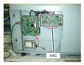
**3.** Remove the six screws securing the board and remove AAC.
