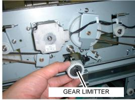
**2.** Remove the shaft's E-ring and remove the bearing.
