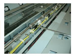
**3.** Remove PSS09 by unplugging the connector and unscrewing the bracket screw.
