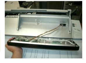
**3.** Remove one cable clamp securing screw.
