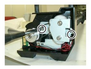
**2.** Remove the screws at the two locations shown in the photos.
