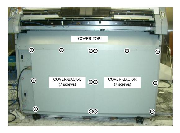
To remove the screws on top of the COVER-TOP, open the fuser unit drawer and insert the screwdriver from the top.
