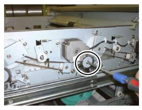
**3.** Remove the GEAR LIMITTER behind the scale.
