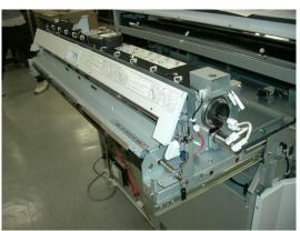
**14.** Remove the plate with two screws at the location shown in the photo.
