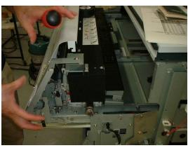
(c) Remove the plate at the location shown in the photo (both right and left).
