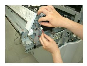
**5.** Remove the SL01 with two screws along with the bracket.
