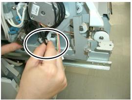
**7.** Remove the plate with two screws at the location shown in the photo.
