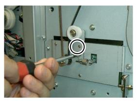
**5.** Remove the motor bracket with three screws.
