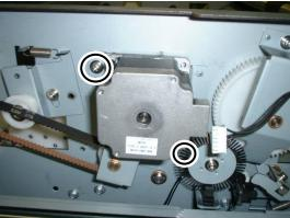
**4.** Remove the MOTOR FM with two screws.
