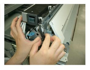
**10.** Remove the TORQUE LIMITER with the gear.
