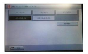
7. The central part of the LED head lights red for several seconds. Check visually that the LED head lights up.
