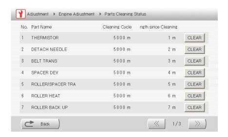
Table 2-16 Parts for Cleaning and Cleaning Cycle
