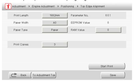
Selecting Print Length, Paper Width, or Paper Type displays the EEPROM and RAM values of the corresponding engine control parameters for the top edge lignment.
