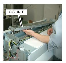
**8.** Remove the CIS UNIT while holding down the center area of the scanner glass.
