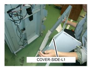
**4.** Remove the plate with the two screws at the location shown in the photo.
