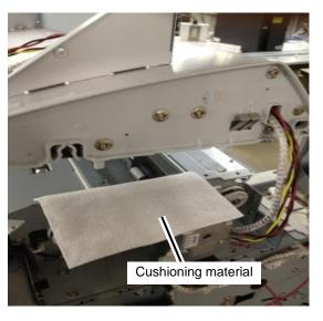
**7.** Remove the FRAME-PINCH-R with seven screws.
