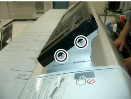
2. Hold both sides of the PANEL ASSY or PANEL ASSY PL PL and pull it out in the same direction as the operation panel surface. Once you have pulled it out, place it down temporarily on the document table.
