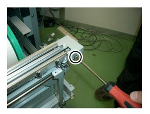
**6.** Pull out the CUTTER UNIT AUTO in an upwards direction.
