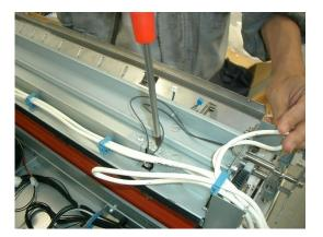
**13.** Remove the TH01, TH02, and TH04 with one screw, from the bracket.
