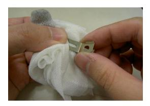
**5.** Apply a thin layer of heatproof grease on the entire PLATE(EARTH).
