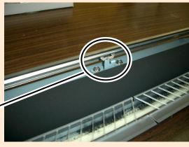
**3.** Remove the HOLDER(TRA-V) with three screws.
