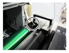
**2.** Grease at the high voltage supply and ground contacts with the process cartridge inside the Printer.
