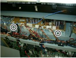
**4.** Pull out the board about half-way, then unplug all connectors at the rear of the board.
