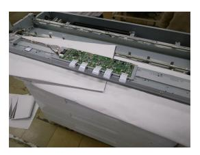
**10.** Remove the CBLS-LVDS clamp with one screw.
