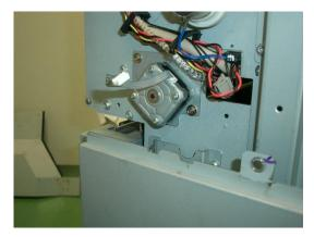
7. Remove the two motor bracket screws.
