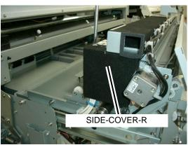
**8.** Release all halogen heater cables from all light blue cable clamps.
