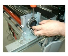
**12.** Remove the HR-WASHER on the right edge of ROLLER HEAT.
