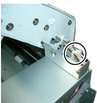
**9.** Remove only one of the screws securing STOPPER-PINCH-UNIT-R, then use the other screw as a pivot point to slide the part over as shown in the photo.
