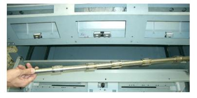
**13.** Remove the TORQUE LIMITTER REGIST from the shaft.
