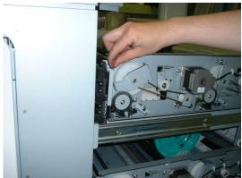
**2.** Remove the plate with two screws above GEAR ONEWAY.
