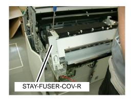
**5.** Remove the COVER-FUSER-L and COVER-FUSER-C4.
