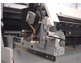
(h) Remove the connector from the solenoid's harness.
