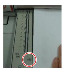
\* To scan in 600 dpi resolution, set the original to the **880** mark on the right of the multifunction printer document table.
