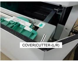
Remove the screws of the right and left brackets fixing the cutter unit. Then move the cutter unit inward as far as it goes.
