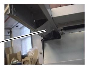
**9.** Remove the SIDE-COVER-L with one screw.
