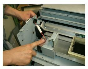
**9.** Remove the stopper with the two screws on the left side of the DEVELOPER UNIT.
