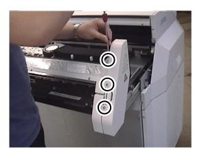
(d) Remove the COVER-FUSER-C3 with two screws.
