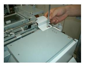
**4.** Remove the plate with two screws from the right side of the Printer at the location shown in the photo.
