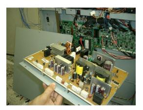
**6.** Remove the securing screw and remove HE RELAYS from the location shown in the photo.
