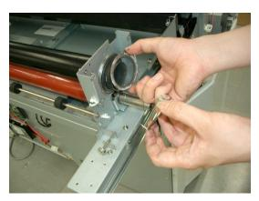
13. Remove the bearings on the right and left of ROLLER HEAT.
