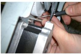
**3.** Also remove the E-ring on the other side of the shaft, then remove the bearing.
