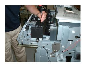
(f) Loosen the EXTENSION-PAPER OUT-KIT(MID)'s four securing screws (two on the right and two the left).
