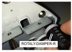
**6.** Lay cushioning material to prevent damage to the shading guide, and place the SC-TOP-COVER as shown in the picture.
