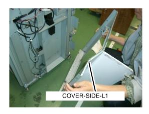
**4.** Remove the plate with the one screw at the location shown in the photo.
