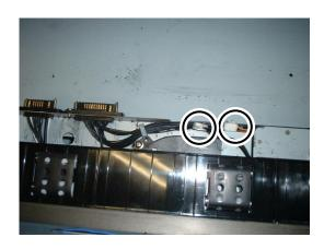
**3.** Remove the two screws at each end of the unit.
