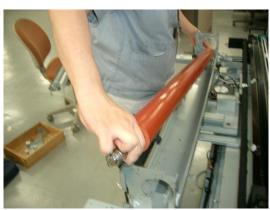
**4.** Remove the JIKUUKE(BR) on both edges of the ROLLER BACK UP ST.
