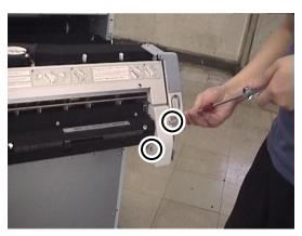
(f) Remove the STAY-FUSER-COV-R with two screws.
