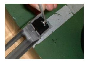
**3.** With a set of tweezers remove the spring-side ring, and remove the WIRE(CHARGER).
