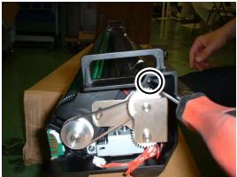
**3.** Cut the cable tie and unplug the connector.
