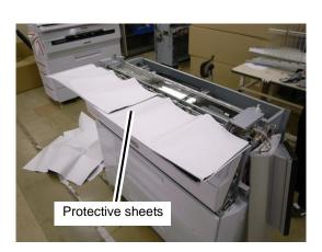
7. Lift up CIS UNIT, starting with the left side first
