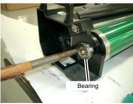
**7.** Remove the bearings on the opposite side (the wheel train side).
