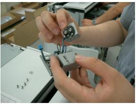
**7.** Remove each sensor with two screws from their respective stay.
