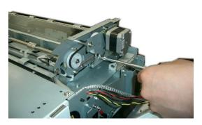
(b) Move the loosened screw to the right side of the guide and tighten it temporarily.
