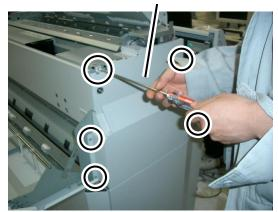
(d) Loosen the screw securing the nip on both the right and the left.
