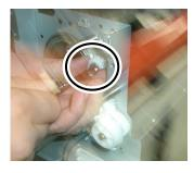
**11.** With a precision screwdriver, remove the PLATE(EARTH) with three screws on the right edge of ROLLER HEAT.
