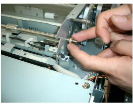
**7.** Remove the E-ring and bush from the left side of ROLLER SC ASSY shaft.
