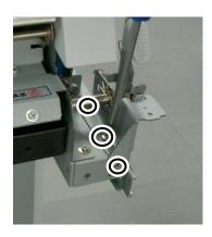
**7.** Remove the two screws shown in the photo.
