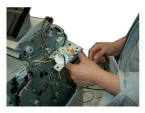
**8.** Remove the MOTOR SC with two screws from BRACKET-MOTOR-SC.
