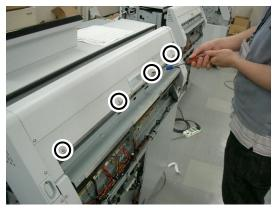
2. Remove the outlet cover with four screws.
