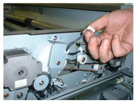
**3.** Remove the bracket with MOTOR FM installed, with two screws.
