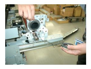
**10.** Remove the E-rings and gears at the location shown in the photo so that you can remove the bearings in step 12.
