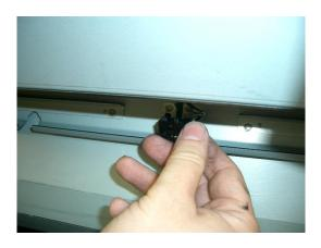
**3.** Pinch the clamp on the back side of the PS16 and pull it out towards you.
