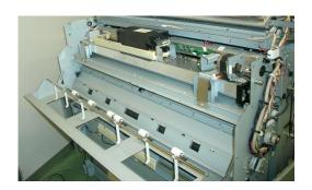
**7.** Remove the plate spring with the four screws and the plate with the four screws, shown in the photo.
