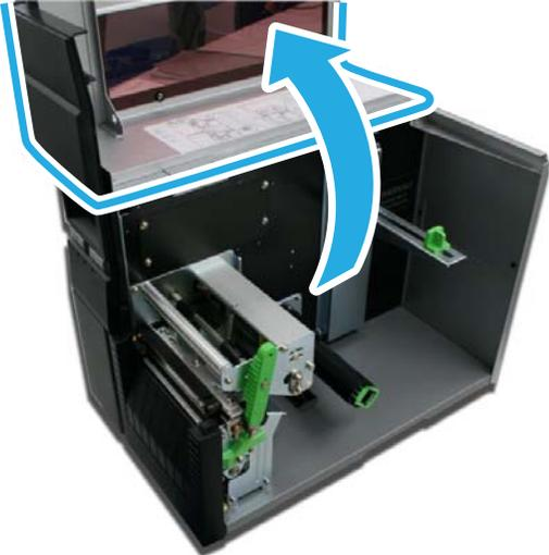
2. Open the printer front door: push down on the green dispenser latch (1) to release the door, then swing it open (2).
