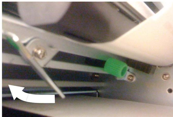
9. Swing the Head Latch back down to close the print head, then latch it in place.
