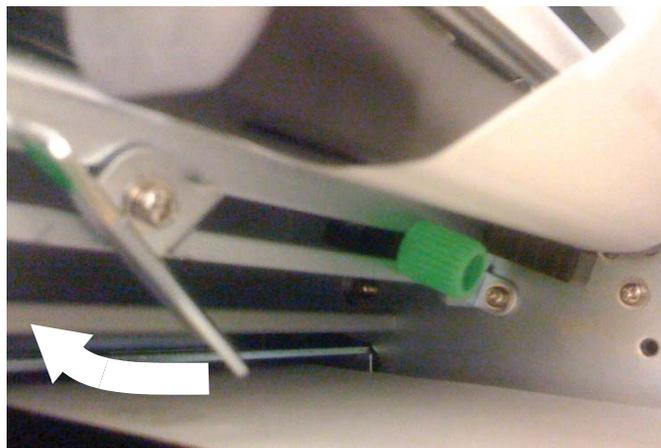
10. Pull the media roll out until about 24 inches are exposed, then remove the labels from that section. Feed the end of the liner back into the bottom of the printer, under the Backing Drive Roller (1).
