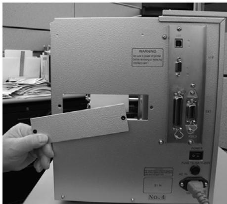
3. Place the stack of fanfold media behind the printer and feed the first label in through the opening.
