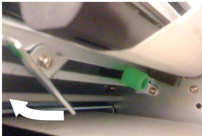
10.Swing the Head Latch back down to close the print head, then latch it in place.
