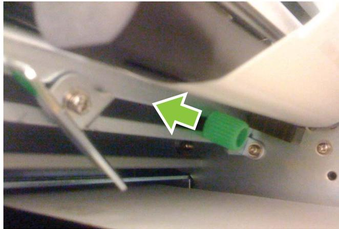
8. Pull out the bottom of the Outside Media Guide so that it is upright, then push the guide inward until it barely contacts the outside edge of the media.
