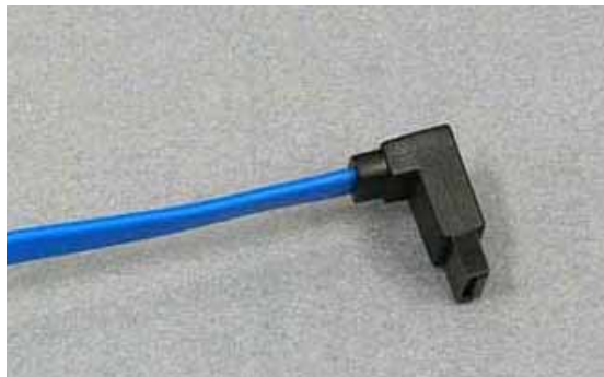
Fig. 5: Connect the right-angle connector to the main board's SATA4 (blue) connector
