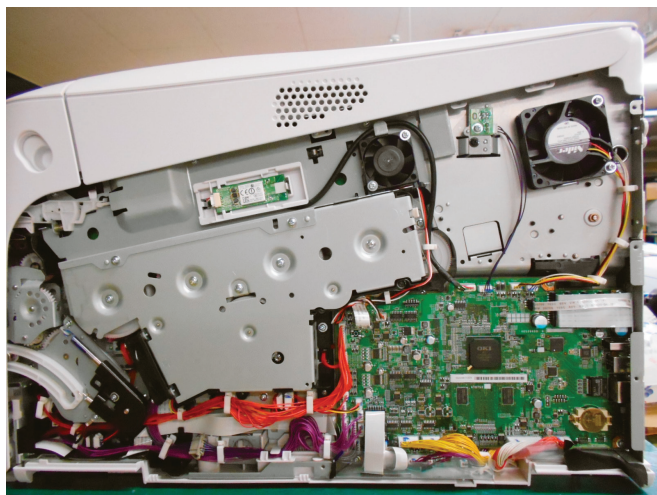
Cable Route picture of around of the CU/PU board.
