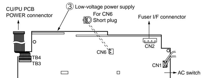
**Note!** CN6: A connector used to switch the AC input voltage setting
