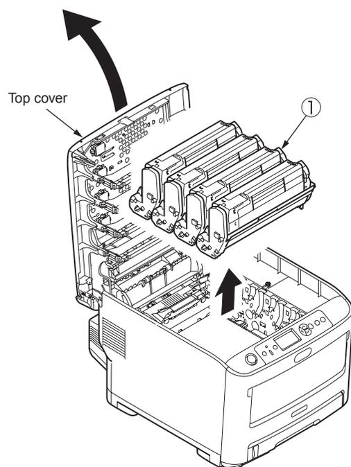
**Note!** Cover the removed image drum cartridge with black paper.
