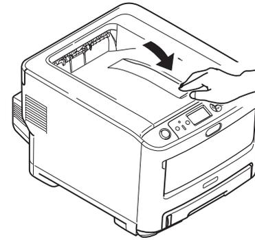
**Note!** If the message of [%COLOR% Waste Toner Full.Replace Toner.] on the control panel doesn't disappear indefinitely, please make sure that the lever of the toner cartridge is fully moved in the direction of the arrow.
