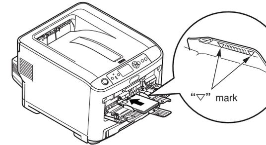
**Note!** Set papers so that paper should not exceed the "▽" mark. (100 sheets of paper with ream weight of 70 kg or 10 envelopes)
