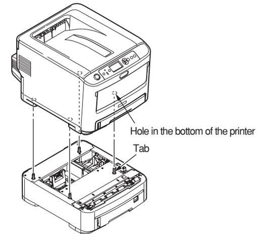
**Note!** When you install two optional trays to the printer, set the optional tray directly on top of the other optional tray, and then put them on the printer.
