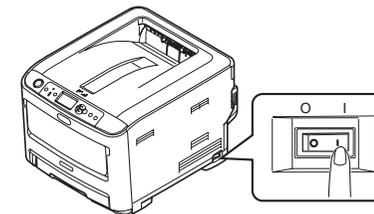
If the printer is completely started up, the message "Ready To Print" would be displayed on the control panel shown as follows.
