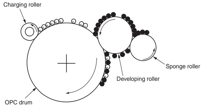
2. The electrostatic latent image on the surface of the OPC drum surface is visualized by toner.
