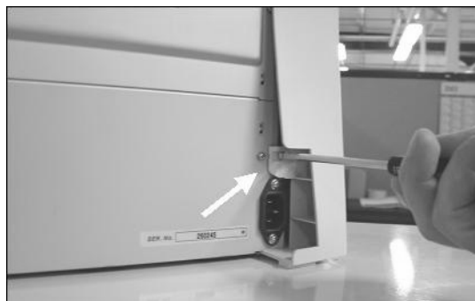
Mounting screw of left-hand side cover
