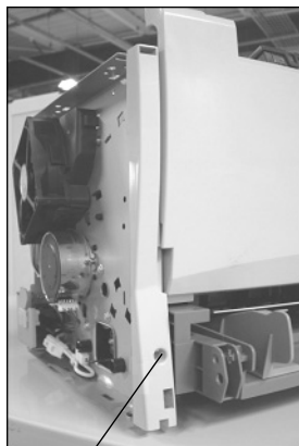
Mounting screw of the left-hand side printer cover
