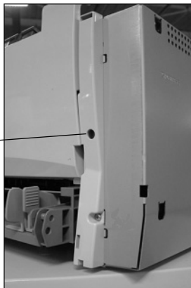
CPU module mounting screw
