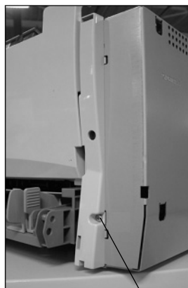
Mounting screw of the right-hand side printer cover
