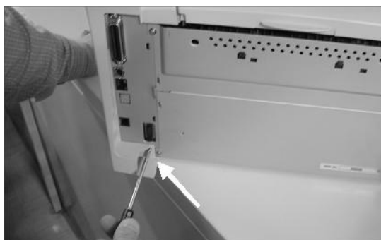
Mounting screw of right-hand side cover
