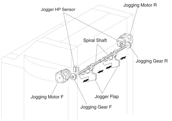
The Jogging Motor transmits a driving force to the Jogging Gear. The rotation of the Jogger Gear rotates the Spiral Shaft. Then, the Jogger Flap moves on the Spiral Shaft.
