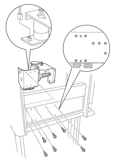
Drive Assembly-ELEV, Motor Assembly-MD11 Removal
