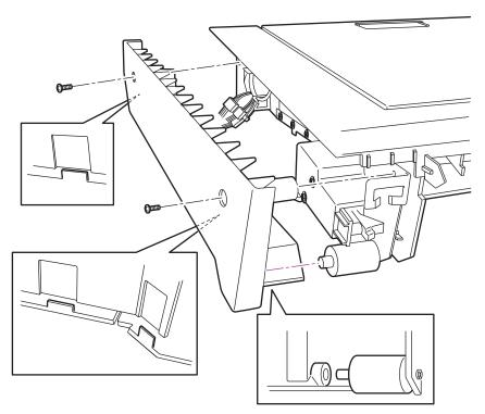
• Remove two screws that secure the Rear Cover to the H-Tra, and then remove the cover.
