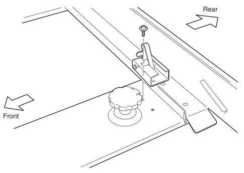
Remove the screw that secures to the Rail from the Lever Assembly, and remove the Lever Assembly.
