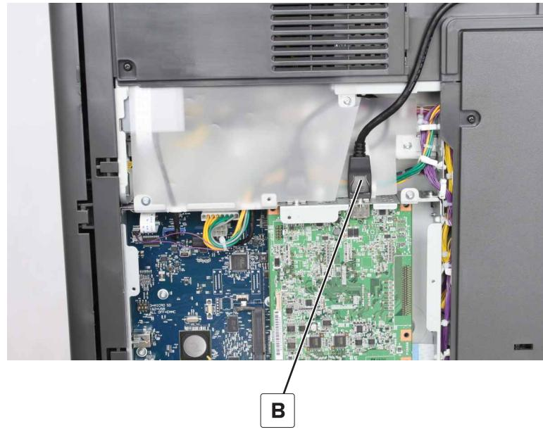
**Installation note:** Connect the scanner CCD cable (A) and ADF CIS data cable (B) as shown in the illustration. If the cables are connected to the wrong socket, then an invalid scanner code error occurs.
