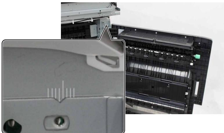
2 Remove the two screws (A), and then remove the upper hinge.
