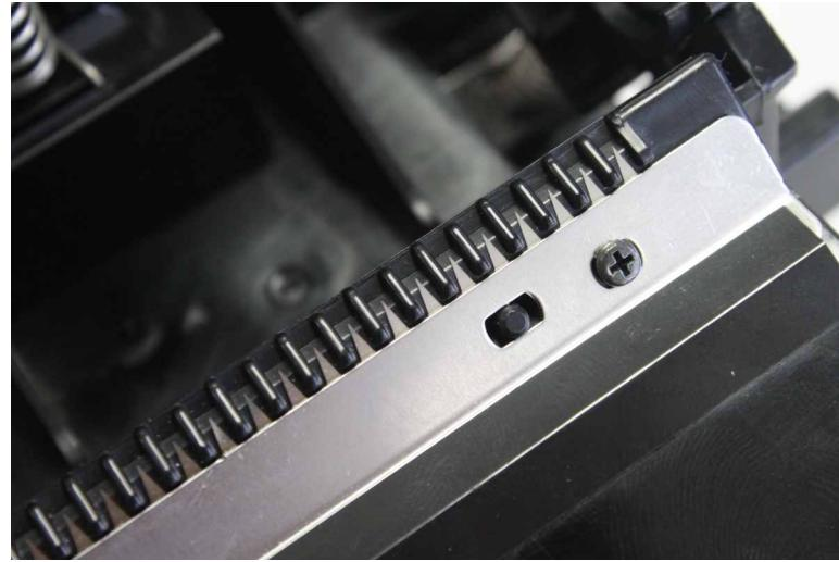
**Installation note:** Align the two springs while pushing down the assembly, and then move the assembly to the left to lock.
