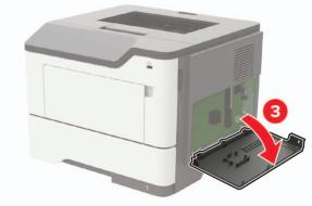
**3** Position the printer on its left side, and then remove the screw (A).
