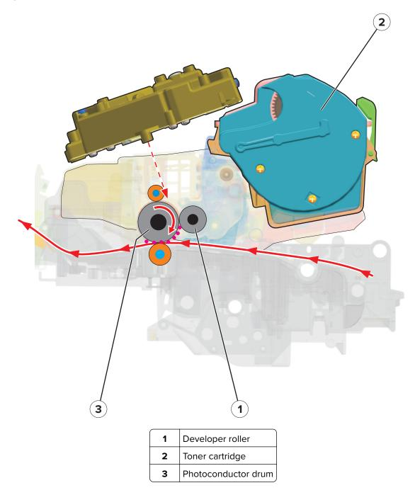
The developer unit applies the toner from the toner cartridge to the photoconductor drum. The difference in charge causes the toner particles to attract to the photoconductor drum areas which are exposed to light.
