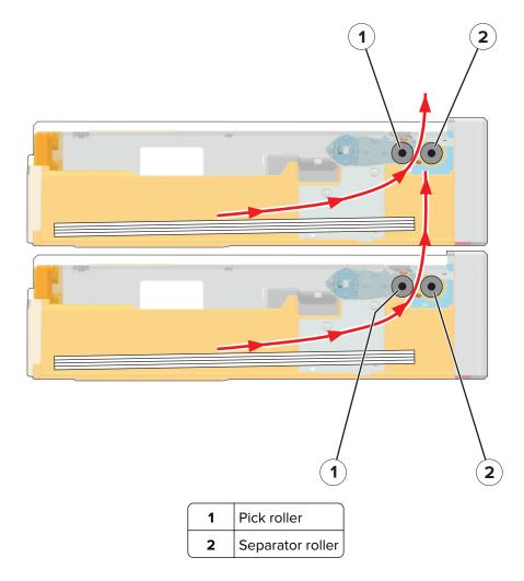
To prepare for feeding, the lift plate raises to push the paper against the pick roller. The lift plate stops pushing at the point where the pick roller is at the proper height for picking. After the pick roller is in position, it feeds the topmost paper to the separator roller. The separator roller rotates in a direction opposite to the pick roller to ensure that only one sheet is fed at a time.
