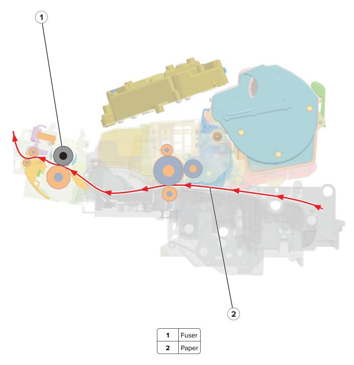
Even if the toner image is already on the paper, the toner particles are not yet permanently bonded to the surface. For the final part of printing, the paper is transported to the fuser where heat and pressure are applied to it. As a result, the toner particles melt and permanently fuse with the paper, completing the print process. The print cycle repeats for the succeeding pages.
