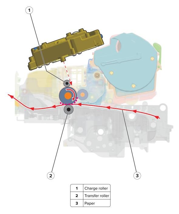
The transfer roller applies a positive charge to the paper, which is pressed between the transfer roller and the photoconductor drum. Due to relative opposite polarities between the paper, from the transfer roller, and the photoconductor drum, from the charge roller, the charge attracts the toner onto the paper.
