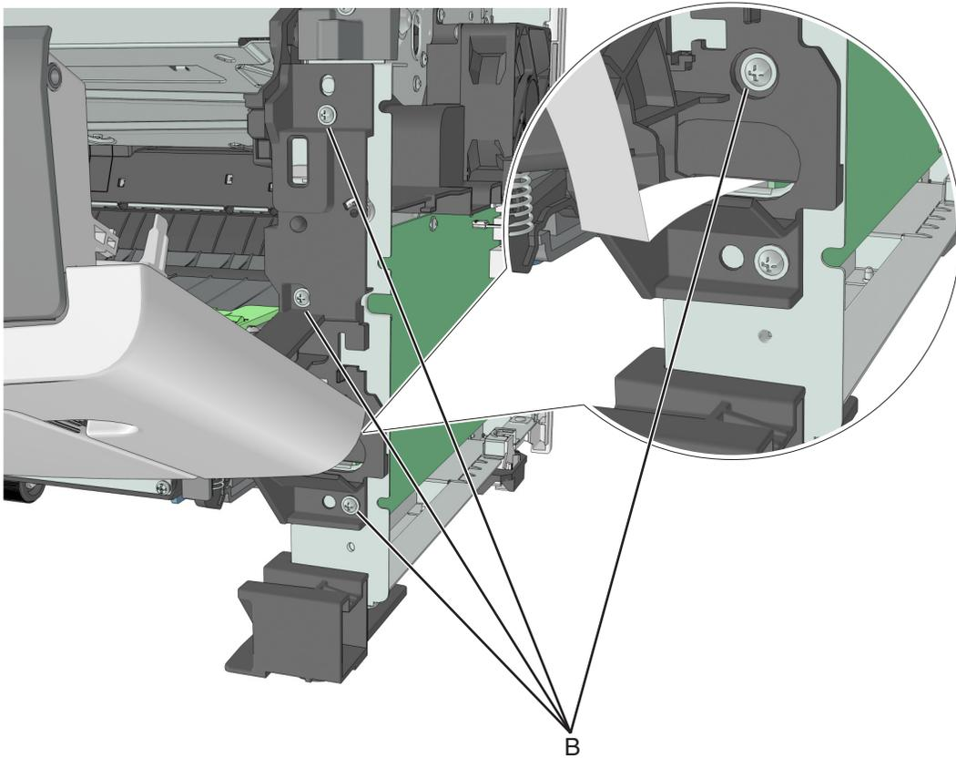
**6** Remove the right front mount, and then remove front door.
