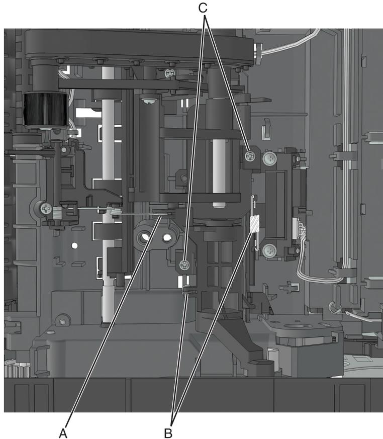
Below are the cam release and bracket.
