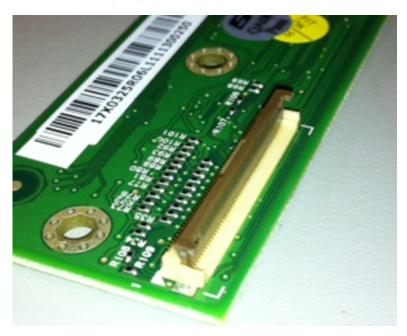
2 Insert the cable below the actuator with the contacts facing downward and away from the locking actuator.Note: Make sure that the cable is installed squarely into the connector to avoid intermittent failures.
