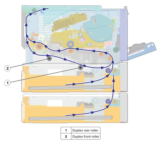
After the first side is printed, the paper is diverted to the top of the paper exit roller. The duplex path opens, and then the paper reverses direction to get its opposite page printed.
