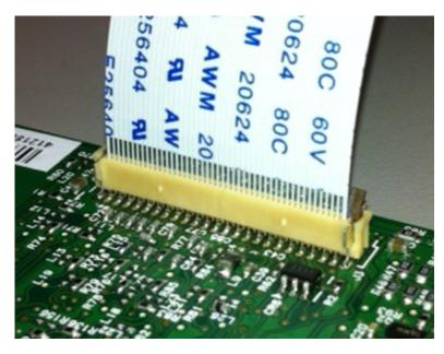
**3** Rotate the locking actuator to the locked position.
