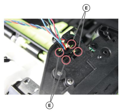
**8** Remove the toner cartridge smart chip contact.
