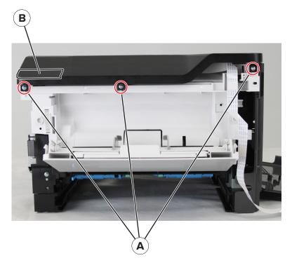
**4** Remove the control panel assembly.
