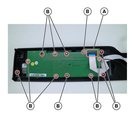
**3** Remove the cover, buttons, and board.
