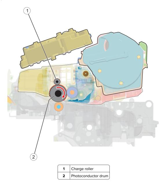
A uniform negative electrical charge is applied by the charge roller to the surface of the photoconductor drum. The photoconductive properties of the surface material allow it to hold the charge as long as it is not exposed to light.
