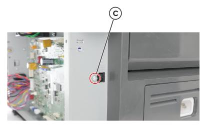
**5** Remove the controller board.
