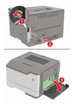
**3** Position the printer on its left side, and then remove the screw (A).
