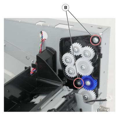
**6** Remove the redrive gear plate.
