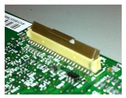
2 Insert the cable on top of the actuator with the contacts facing away from the locking actuator.Note: Make sure that the cable is installed squarely into the connector to avoid intermittent failures.
