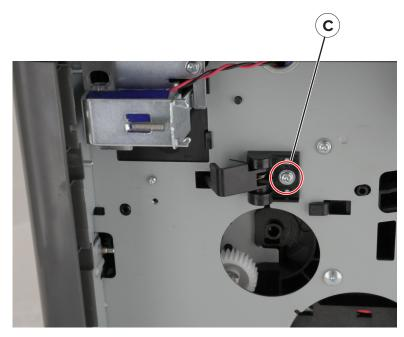
**5** Remove the fuser actuator.
