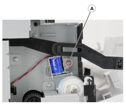
**3** Cut the cable, and then remove the solenoid.
