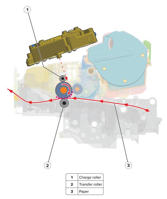
The transfer roller applies a positive charge to the paper, which is pressed between the transfer roller and the photoconductor drum. Due to relative opposite polarities between the paper, from the transfer roller, and the photoconductor drum, from the charge roller, the charge attracts the toner onto the paper.
