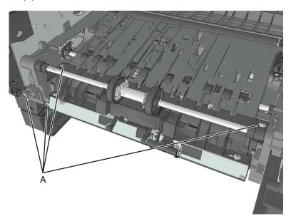
**8** Push and hold the cam restraint to release the MPF shaft.
