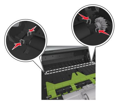
**2** Lift to remove the transfer roll.
