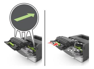
**8** Insert the toner cartridge by aligning the side rails of the cartridge with the arrows on the side rails inside the printer, and then insert the cartridge into the printer.
