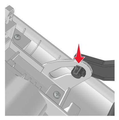
**5** Remove the screw (A) to disconnect the ground wire.
