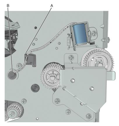
**d** Route the cable using the new path, and secure it with a cable tie (C).
