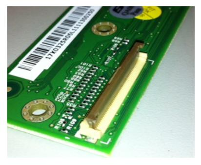
2 Insert the cable into the ZIF connector with the contacts facing downward and away from the locking actuator. The cable needs to be inserted below the actuator.
