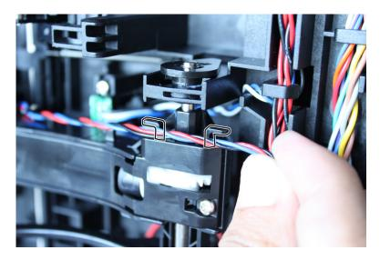
${f d}$  Loop the cable behind the right cable holder.
