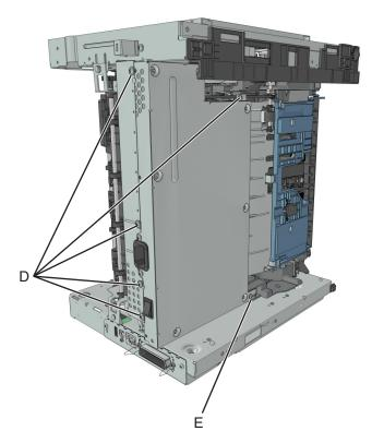
**7** Remove the power supply, and then disconnect all cables from the power supply.
