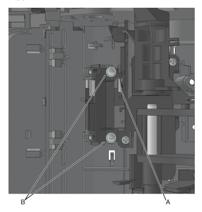
**9** Disconnect the cable from the sensor.
