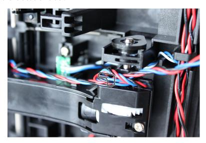
**g** Pull the free end to make sure that the cable is tightly looped around the cable holders.
