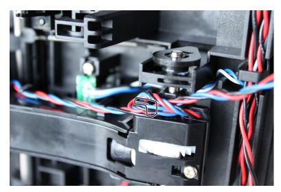
**g** Pull the free end to make sure that the cable is tightly looped around the cable holders.
