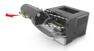
**3** Lift the green handle, and then pull the imaging unit out of the printer.
