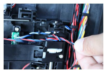
**h** Route the cable using the new path, and secure it with a cable tie (A).
