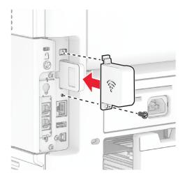
Close the controller board access cover, and then install the screw.
