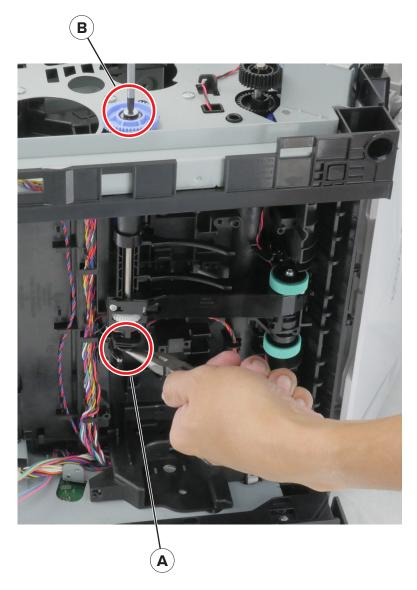
Pull out the pick roller clutch, and then cut the cable to remove it.
