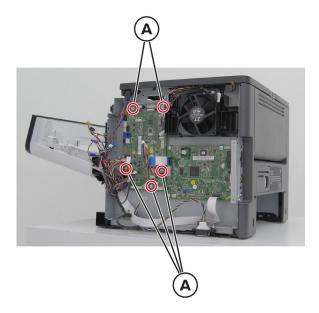
Remove the engine board.
