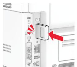
Attach the wireless print server cover, and then install the screw.
