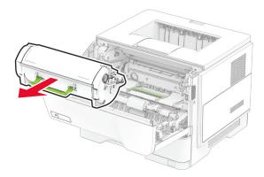
**3** Remove the used imaging unit.
