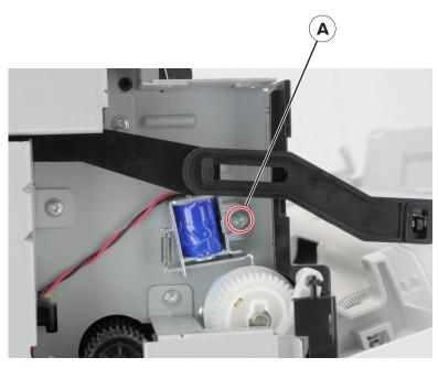
**3** Cut the cable, and then remove the solenoid.
