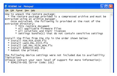
**6** If the printer had eSF apps previously installed, then confirm from the customer if all the eSF apps have been installed after performing the installation instructions in the *Readme* file.
