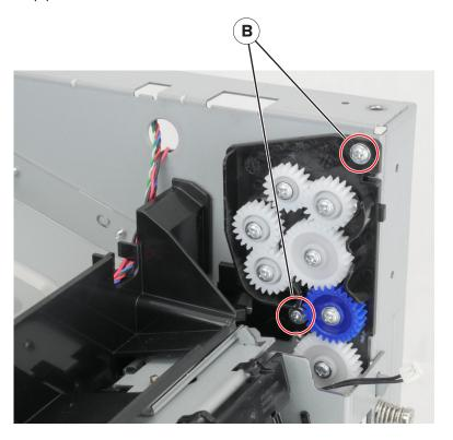
**6** Remove the redrive gear plate.
