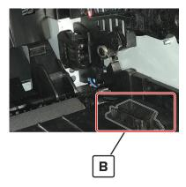
**4** Check the imaging unit for damage, contamination, and improper installation.
