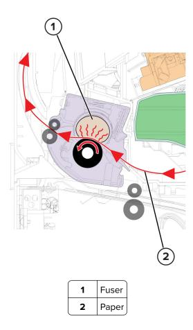
Even if the toner image is already on the paper, the toner particles are not yet permanently bonded to the surface. Paper is transported from the transfer roller to the fuser where heat and pressure are applied to it. As a result, the toner particles melt and permanently fuse with the paper, completing the print process. The cycle repeats for the succeeding pages.
