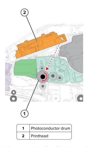
The printhead laser emits the light that contacts the surface of the photoconductor drum. An invisible image, called *digital latent image*, is written as the light turns on or off. The light causes areas of the photoconductor drum surface to lose charge, resulting in a relative opposite polarity.
