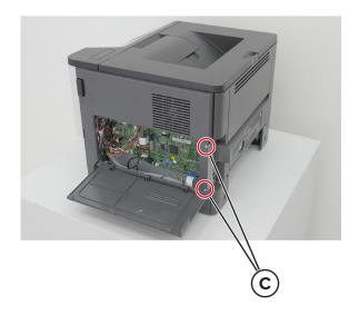
Place the printer on its left side, and then remove the right cover.
