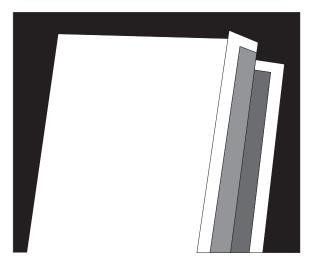
**5** If the grid lines of the right flap align below the corresponding lines on the left side, then adjust the printhead clockwise relative to the printer, and recheck. If the grid lines of the left flap align below the corresponding lines of the right side, then adjust the printhead counterclockwise.
