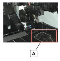
**4** Check the power supply for damage, contamination, and improper installation. For more information, see <u>"Power supply removal" on page 208</u>.
