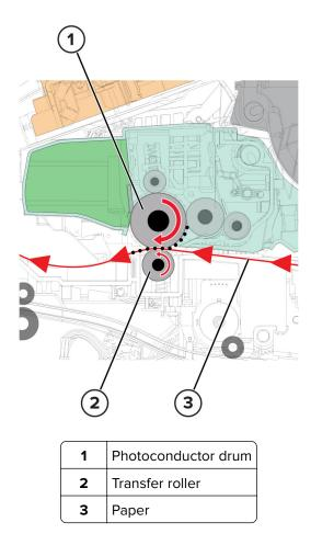
The transfer roller applies a positive charge to the paper, which is pressed between the transfer roller and the photoconductor drum. The charge on the paper received from the transfer roller is positive. The charge on the photoconductor drum received from the charge roller is negative. The relative opposite polarities between the two charges result in the charge attracting the toner onto the paper.
