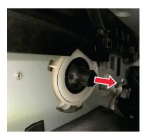
If the couple is stuck, then reach inside the printer and manually reposition the coupler as shown.
