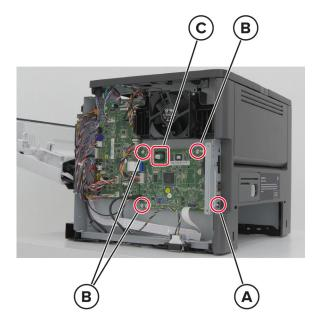
**6** Remove the controller board.
