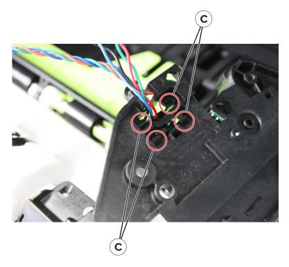
Remove the toner cartridge smart chip contact.
