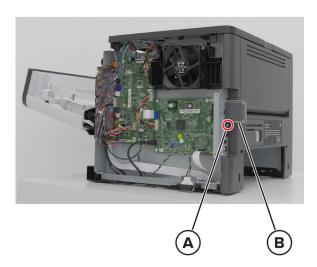
Release the wireless module from the guide, and then remove it.
