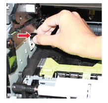
**5** Check if the imaging unit contact (A) is bent, damaged, or not in proper contact with the imaging unit.
