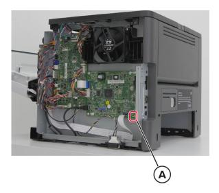
**4** Move the jumper to cover the middle and exposed prongs.
