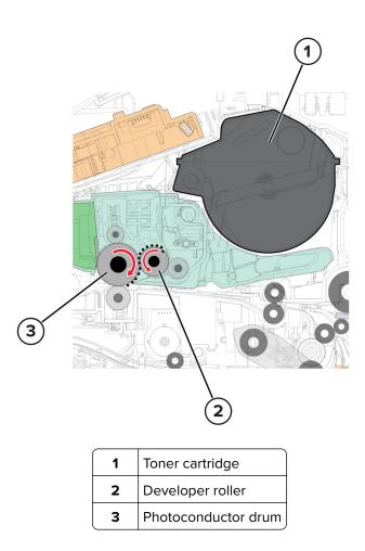
The developer roller applies the toner from the toner cartridge to the photoconductor drum. The relative opposite polarity in charge causes the toner particles to attract to the photoconductor drum areas which were exposed to light.
