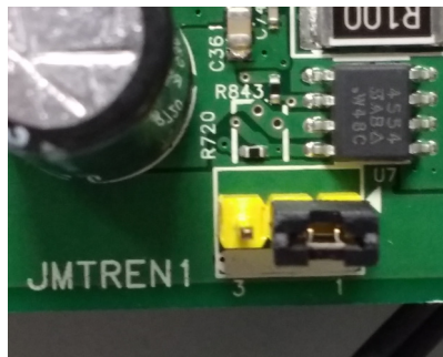
Interlock bypass enabled
