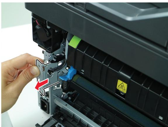
**10** Press the latch. Lock the latch position using a prying tool or screwdriver.
