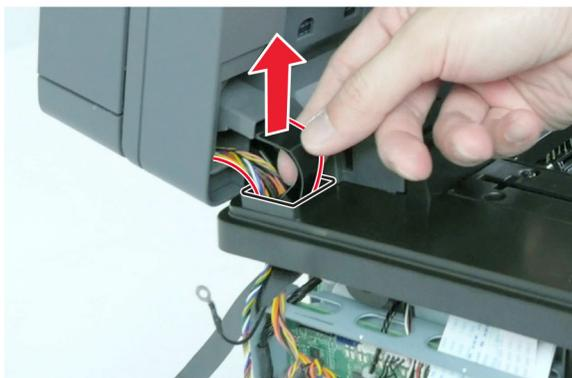
**7** Detach the hinge, and then remove the scanner.
