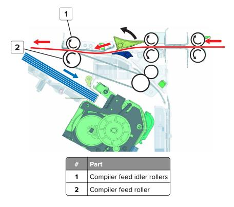
While the first stack is being aligned, the compiler feed roller rotates in reverse and then feeds the paper to the pre-feed guide.
