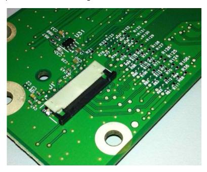
2 Insert the cable on top of the actuator with the contacts facing away from the locking actuator.
