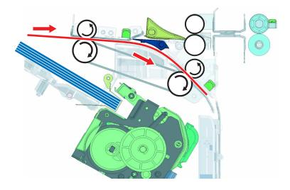
The idler rollers raise, and while the first stack is being stapled, the second sheet is positioned over the first sheet.
