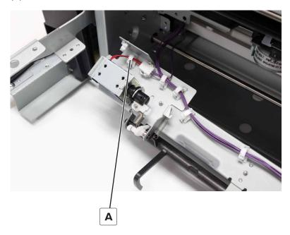
**5** Remove the two screws (B), and then remove the solenoid.
