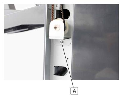
**8** Remove the gear from the bracket.
