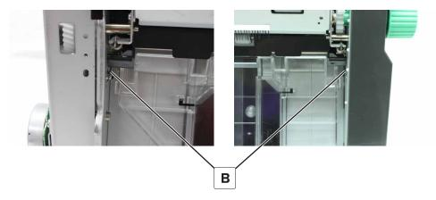
**3** Pry the rear hinge, and then remove the door.
