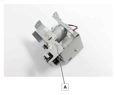
**4** Remove the sensor from the bracket.
