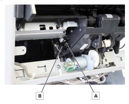
**7** Disconnect the cable from the sensor.
