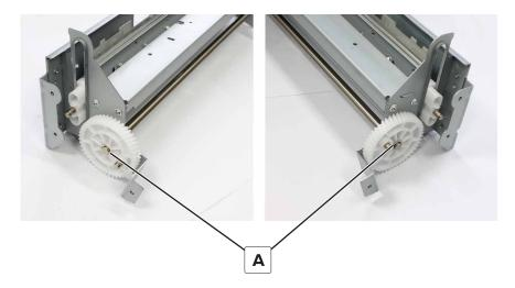
**Installation note:** Align the protruding shafts on each gear with each other.
