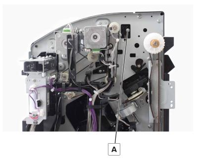
**4** Remove the sensor, and then disconnect the cable.
