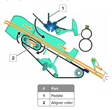
The third sheet is fed over the stack, and then the aligner paddles push the third sheet to the aligners. Succeeding sheets are individually fed and aligned in the same manner as the third sheet.
