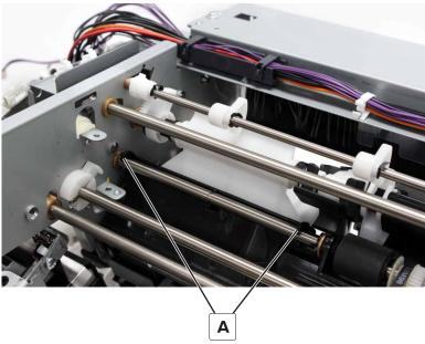
**Installation note:** Position the guides under the flaps (A).
