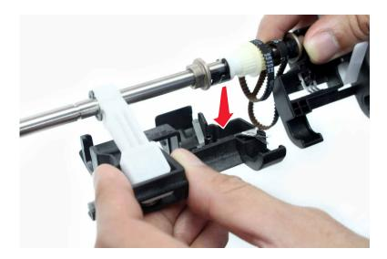
**Note:** Take note of the original position of the ground and the two concentric springs.
