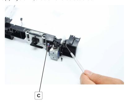
**Installation note:** Take note of the spring position and cable routing.
