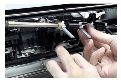
8 Remove the lower exit roller paddles. See <u>"Staple finisher lower exit roller paddles removal" on page 229</u>.
