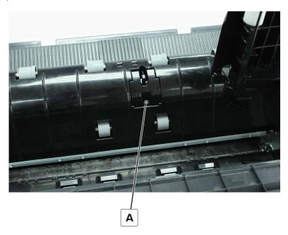
**3** Pry the sensor, and then disconnect the cable.
