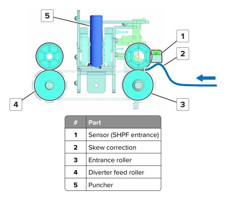
The motor (punch drive) moves the punch unit frames in opposite directions. The motion causes the slots on the frames to move the punchers up and down.
