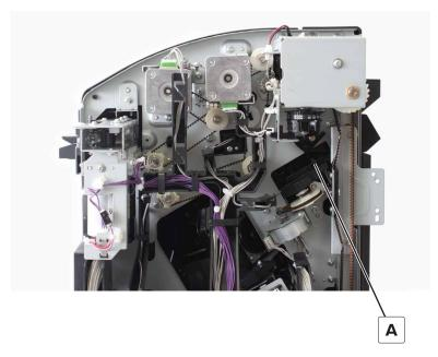
**3** Disconnect the cable from the sensor.
