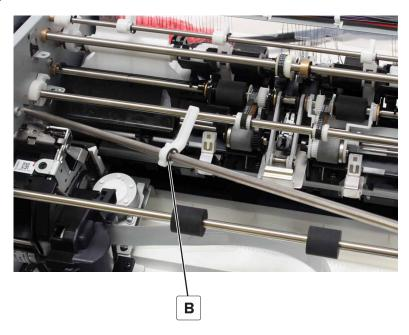
**13** Remove the lever, and then remove the pin.
