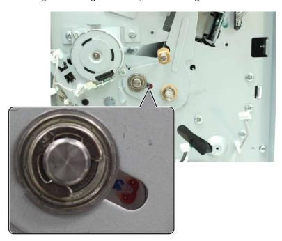
**b** Align the hole on the gear with the hole on the motor bracket.
