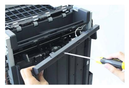
**14** Disconnect the two cables (F), and then remove the guide.
