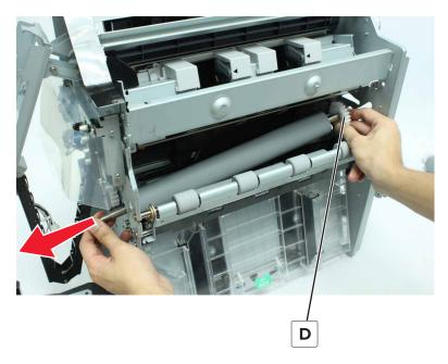
**12** Move the roller to the front. Swing out, and then remove the roller.
