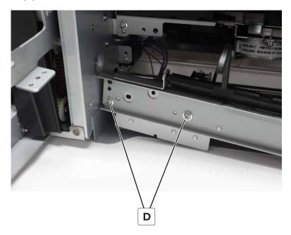
**8** Remove the bracket to release the link from the actuator, and then remove the actuator.
