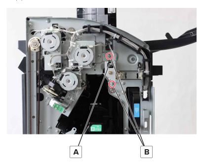
**6** Remove the sensor from the bracket.
