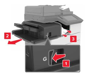
If necessary, turn the spinner wheel G1 downward to feed the jammed paper into the finisher bin, and then remove the jammed paper.
