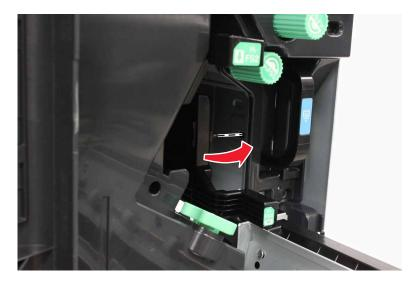
**d** Reach in from the right side, and then pull down the door. The door tabs should set into the holes.
