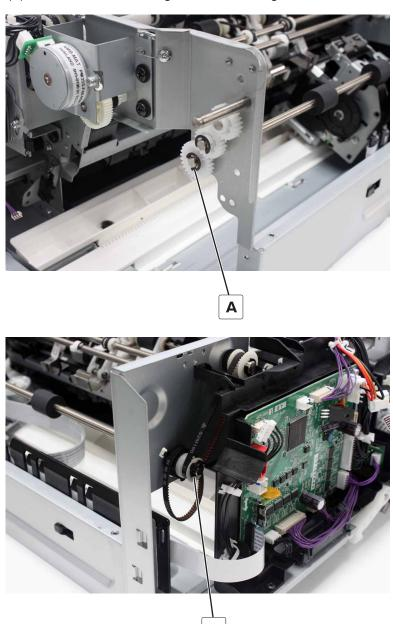
**8** Remove the clip (B), and then remove the shaft.
