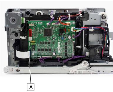
**5** Press the latch, and then remove the cable holder.
