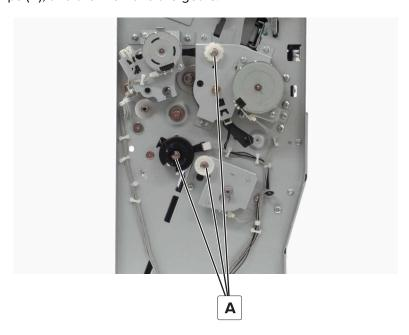
**Installation note:** Align the pointers on the gears with the triangles on the frame.
