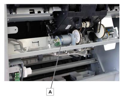
**6** Remove the two screws (B), and then remove the motor.
