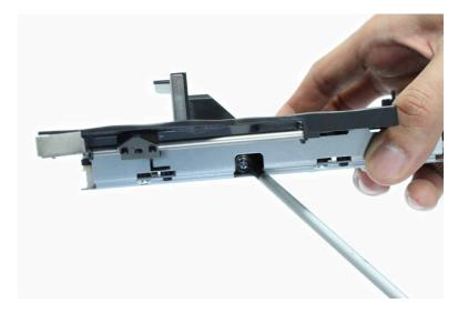
**13** Remove the screw, and then remove the rear tamper.
