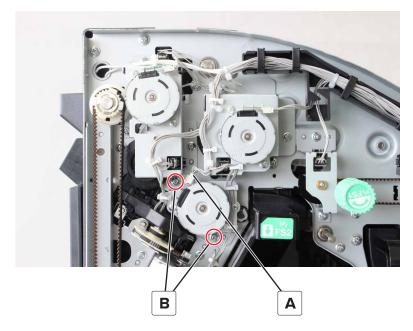
**5** Remove the motor from the bracket.
