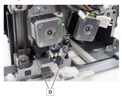
**6** Remove all the cables from the bracket, and then remove the bracket.
