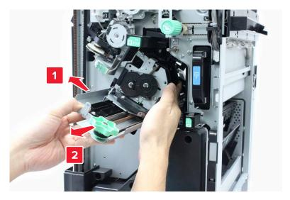
7 Lift the assembly until the cables on the bottom clear the finisher frame, and then remove the assembly.
