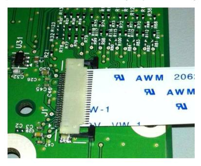
**3** Slide the locking actuator toward the connector to lock the cable.
