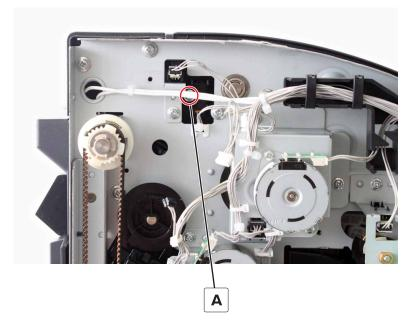
**6** Remove the sensor, and then disconnect the cable.
