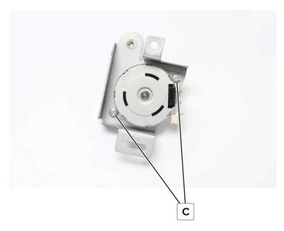
**Installation note:** Rotate the bracket counterclockwise to tighten the belt before installing all the screws.
