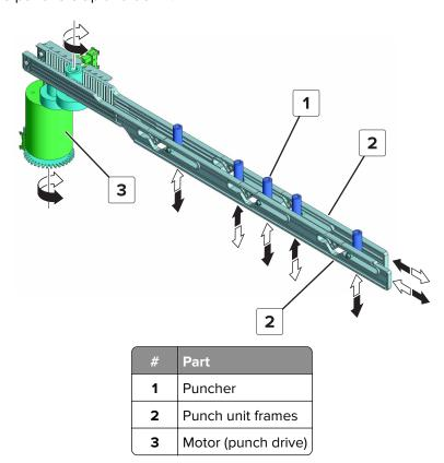
The chad accumulate in the hole punch box below the punch unit. When the light from the sensor (SHPF hole punch box full, transmit) is blocked, the printer determines that the box is full.
