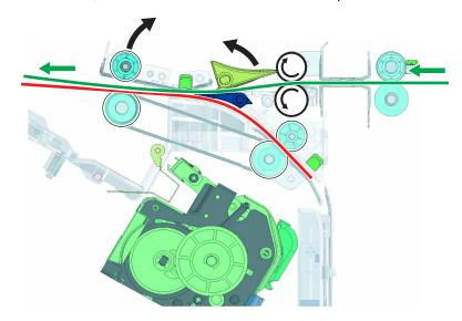
The idler rollers lower, and then the two sheets are fed over the tamper plates. Before the trailing edge passes the compiler feed roller, the tamper plates return to their home position.
