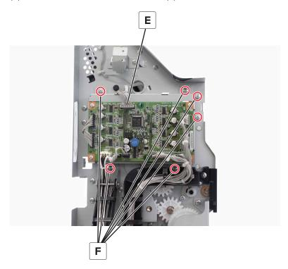
**8** Remove the controller board holder and frame brace.
