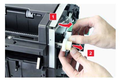
**10** Remove the pin from the shaft.
