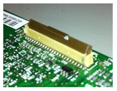
2 Insert the cable on top of the actuator with the contacts facing away from the locking actuator.
