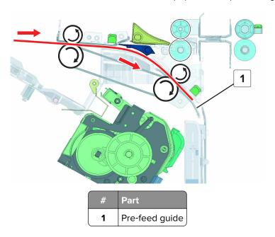
The idler rollers and diverter raise, and then the second sheet is transported over the first sheet.
