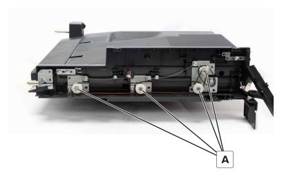
4 Remove the four gears and belts.
