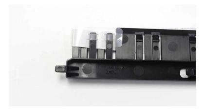
**e** Thread the cable and the film through the rest of the clips.
