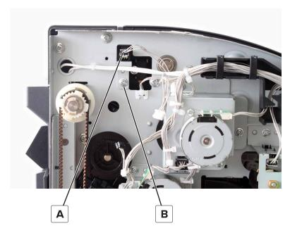
**6** Disconnect the cable, and then remove the sensor from the bracket.
