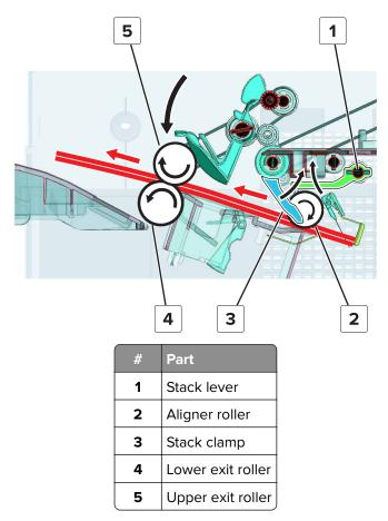
After the trailing edge of the stack passes the exit rollers, the lower exit roller paddles push the edge to feed the stack to the bin. The lower exit roller continues to rotate to return to the home position. The tamper paper present sensor actuator returns to its original position, signaling that the stack is on the bin.
