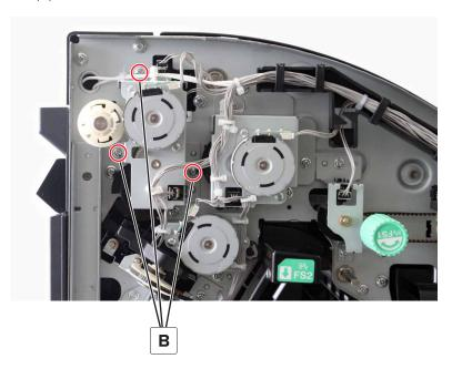
**9** Dislodge the motor bracket from the finisher, and then remove the gear.
