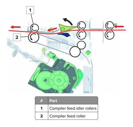
The compiler feed roller rotates in reverse, and then feeds the paper to the pre-feed guide.
