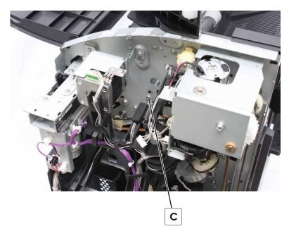
**14** Pry the hinge, and then remove the assembly.
