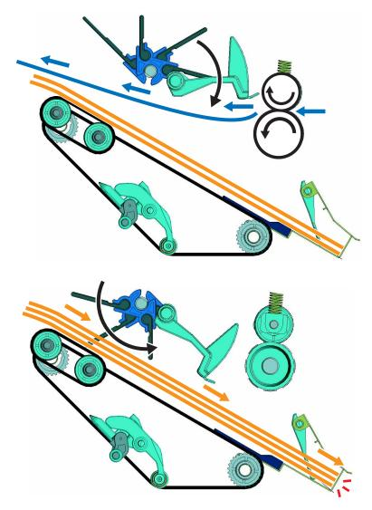
For staple jobs, the trailing edge of the stack is stapled. For two-point staple jobs, the motor (SHPF aligner) drives the aligner shaft to prevent the front and rear aligners from interfering with the staple unit.
