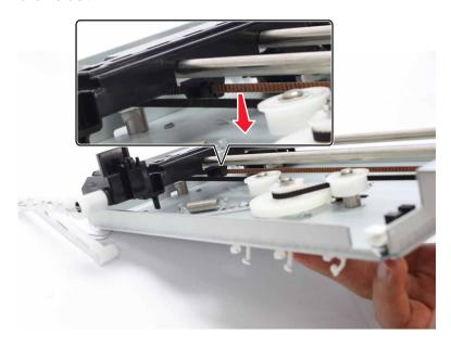
**8** Remove the two clips (A), and then remove the two shafts.
