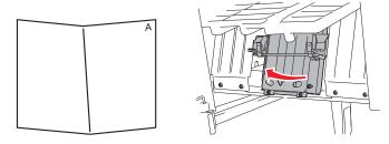
• Rotate the aligner assembly to the front.
