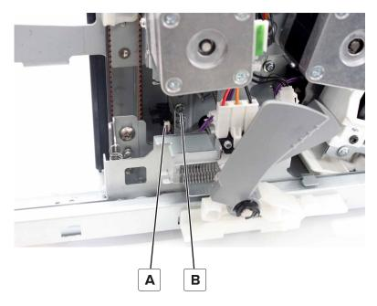
**4** Remove the sensor from the bracket.
