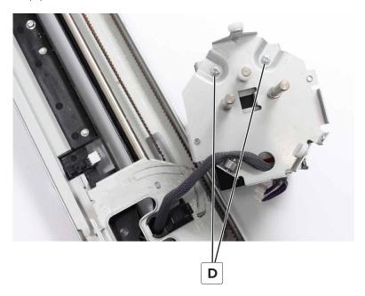
Rotate, and then remove the staple unit.
