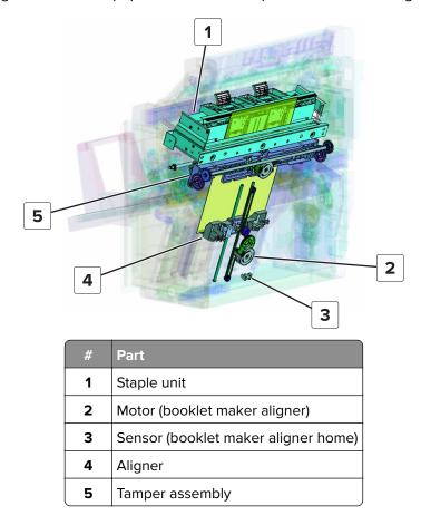
The motor (booklet maker staple unit) controls the stapling process. The paper stack is held between the paper press and clincher for stapling. The stack is then fed to the bifold section.
