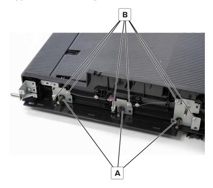
**Installation note:** Position the ground wire over the plates before installing the screws.
