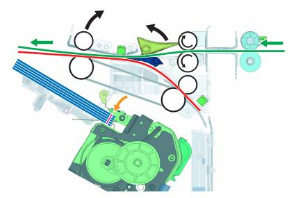
The idler rollers lower, and then the two sheets are fed to the compiler assembly. At the same time, the first stack is fed to the elevator bin. Unlike the first and second sheets, the succeeding sheets of the second stack are individually fed to the compiler assembly.
