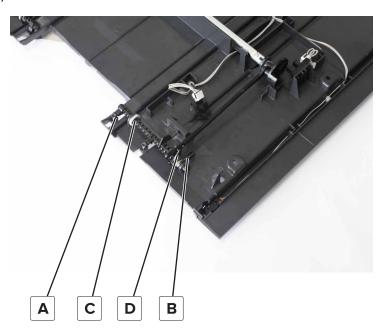
10 Rotate, and then remove the lever.
