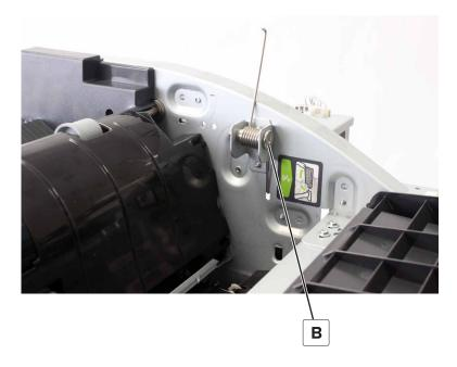
**6** From the door, remove the screw (C), and then remove the spring.
