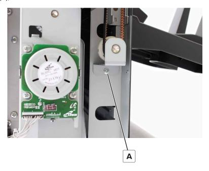
**6** Remove the gear from the bracket.
