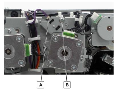
**4** Remove the sensor from the bracket.
