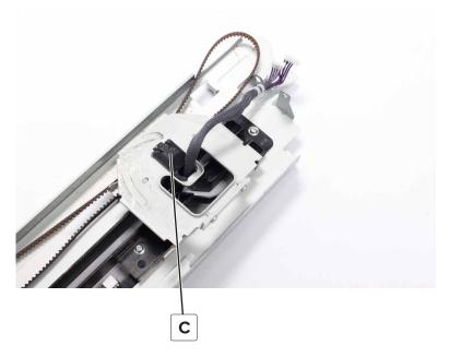
**8** Flip the carriage, and then remove the belt from the holder (D).
