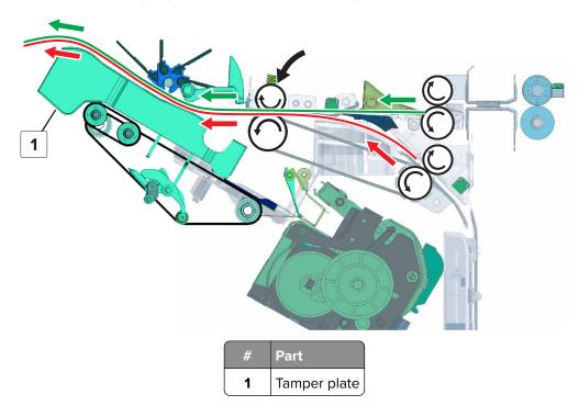
After the trailing edge passes the compiler feed roller, the compiler guide moves down to push down the paper to the compiler assembly. The rotation of the motor (SHPF paddle) and paddle cam control the position of the guide.
