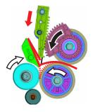
The paper is fed to the trifold roller for the second fold, and then the trifold diverter returns to the home position.
