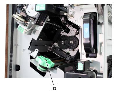
**6** Push the assembly to the left, and then partially pull it out.
