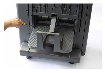
2 Remove the seven screws (A).
