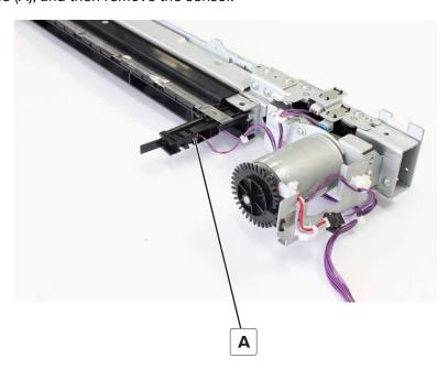
**4** Remove the screw (B), remove the plastic sheet, and then remove the sensor.
