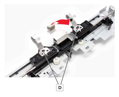
**22** Remove the two ground plates (E) from under the front and rear aligners.
