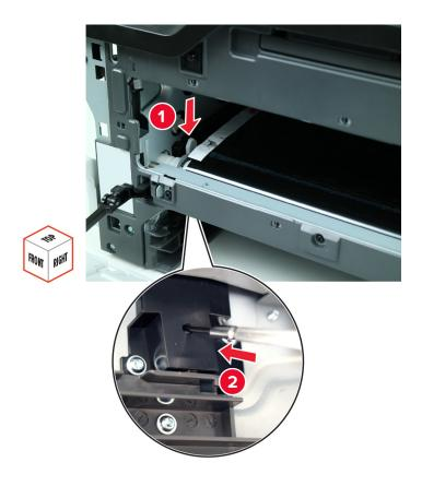
Move the coupler to release the transfer module.
