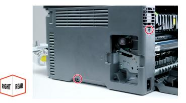
Position the printer as shown, and then release the latches.
