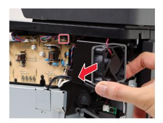
**Installation note:** Stick the pad to the fan on the area shown.
