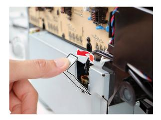
Disconnect all the cables, and then remove the cable screw.
