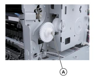
**6** Disconnect the cable, and then remove the clutch.
