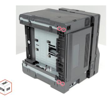
**2** Release the door, and then remove the screw.
