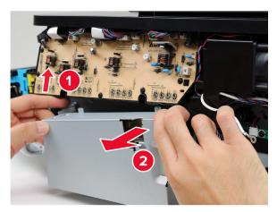
Remove the screw, and then remove the cover.
