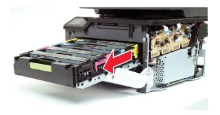
**Warning—Potential Damage:** Extended exposure of the cartridge to light may cause print quality problems.
