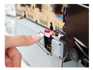
7 Disconnect and release the cables (C), and then remove the screws.
