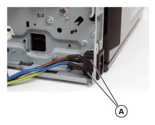
**Note:** Use prying tools to release the remaining latch (A).
