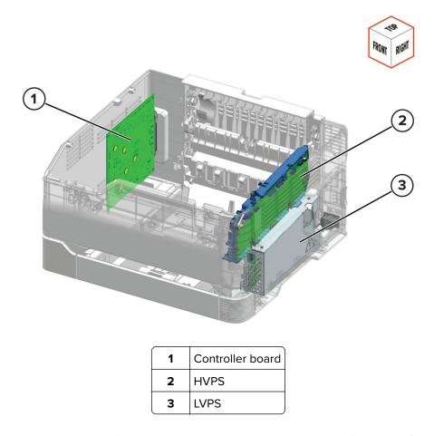
The LVPS (Low voltage power supply) powers the printer. It converts the power from the AC outlet to controlled AC and DC outputs.
