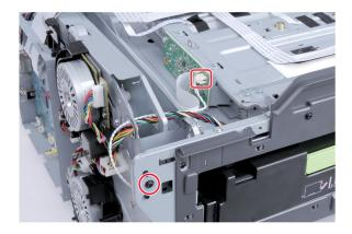
6 Remove the switch bracket.
