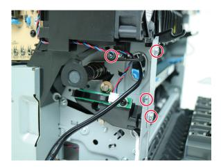
Release the bracket, and then move it out of the way.
