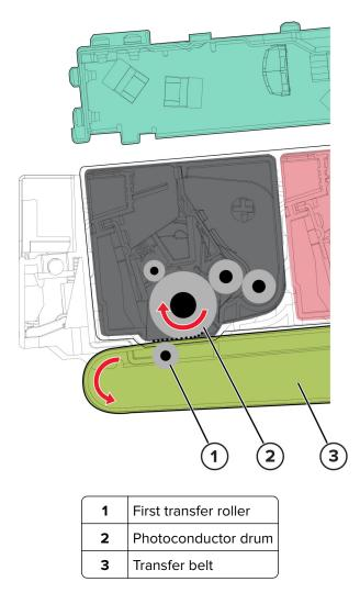
When the latent images are developed on each photoconductor drum, the HVPS sends voltage to the first transfer rollers inside the transfer belt.
