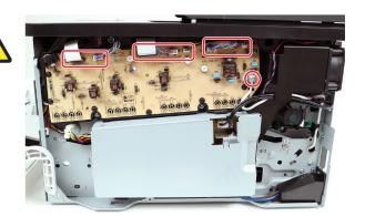
Cut the cable tie, and then remove the screws.
