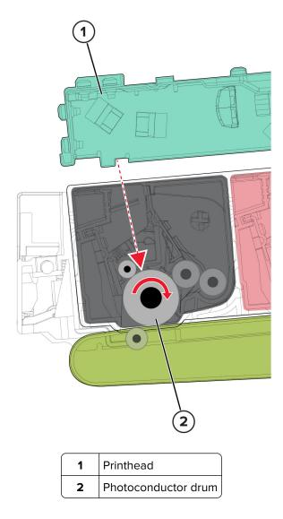
During the expose step, the printhead laser fires a focused beam of light at the surface of each photoconductor drum and writes an invisible image. The image formed for each color is called a *latent image* or *electrostatic image*.
