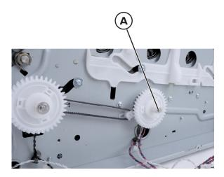
**9** Disconnect the cable, and then remove the clutch.
