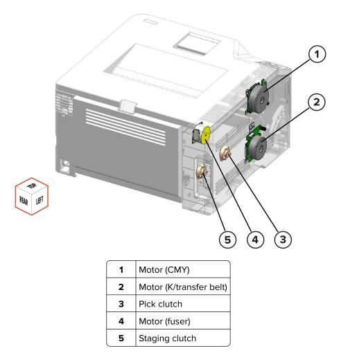
When a print job is sent to the printer, the printhead motor initiates and the fuser starts to heat. After the printhead motor reaches speed, the CMY and K motors begin turning to start the EP process. For more information, see **EP process**" on page 343.
