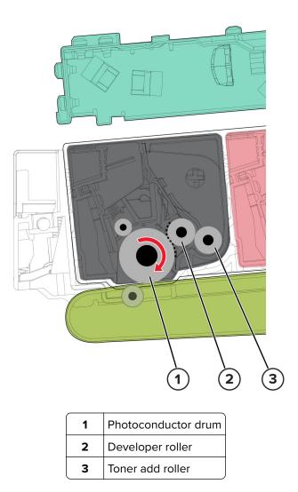
When the laser exposes the photoconductor drum in the print cartridge, the HVPS sends charge to the developer roller. For each color, the print cartridge engages the photoconductor drum so it is in contact with the developer roller. Because of the charge difference, the toner is attracted to areas of the photoconductor drum surface exposed by the laser.
