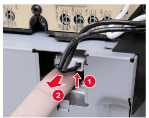
Thread the cable through the hole.
