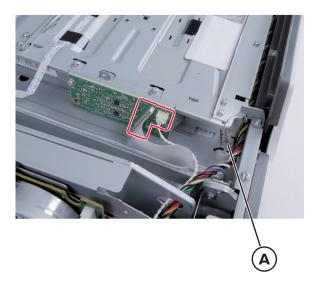
Release the cables from the printhead.
