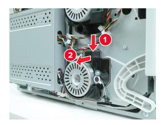
**3** Disconnect the cable, and then remove the screws.
