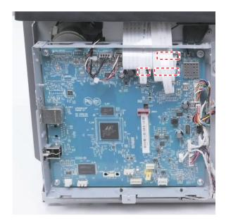
Disconnect the cables and release the spring (A).
