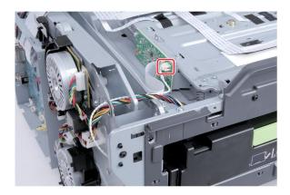
8 Release and thread the cables through the hole (A), and then remove the screws.
