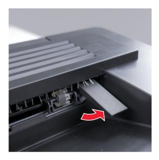
**Installation note:** Move the flag up and down. Check if the flag (A) toggles the sensor. Check if the bin flag drops down freely to its default lower position.
