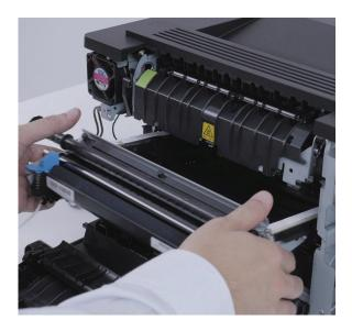
Note: For a video demonstration, see <u>Transfer module removal</u> at infoserve.lexmark.com/ids/sma.
