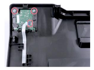
**6** Remove the control panel.
