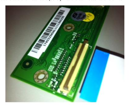
**3** Rotate the locking actuator to the locked position.
