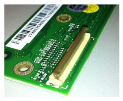
2 Insert the cable below the actuator with the contacts facing downward and away from the locking actuator.
